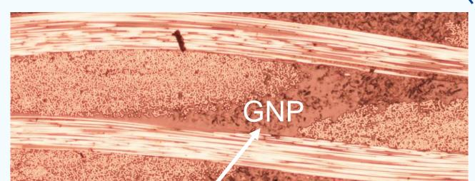
The interpenetrating networks greatly reduced interlayer thermal resistance in the through-plane direction and provided heat transfer pathways other than fibers in the in-plane direction.
