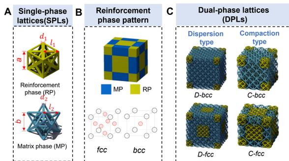
Fig. 1 Architecture design and fabrication of dual-phase lattices (DPLs). (A) Geometrical illustrations of two types of lattice materials, respectively as matrix phase (MP) and reinforcement phase (RP) of DPLs. (B-C) DPLs with bcc and fcc patterns of RP classified as dispersion type and compaction type according to interactions between the reinforcement grains.
