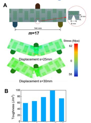
Fig. 5. Toughness simulation models of DPLs. (A) Cracked DPLs in three-point bending. (B) Toughness comparison for DPLs with different RP distribution complexity.
