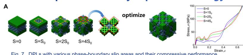
Fig. 7. DPLs with various phase-boundary slip areas and their compressive performance.
