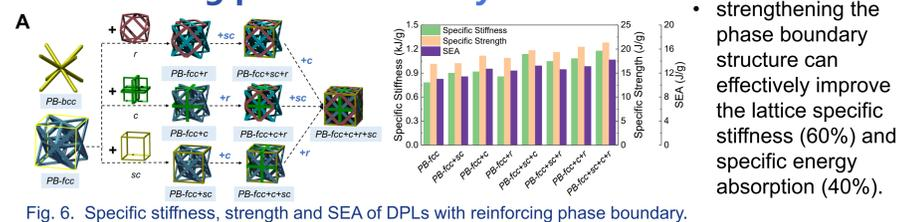
Fig. 6. Specific stiffness, strength and SEA of DPLs with reinforcing phase boundary.
