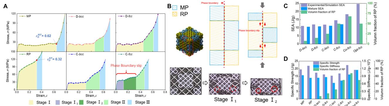
Fig. 3. (A) Compressive stress-strain curves. (B) Illustration of phase boundary accompanying RGs sliding for C-fcc type DPLs. (C) Specific energy absorption (SEA) of DPLs with different volume fractions of RP, compared to results computed from the simple law of mixtures. (D) Specific stiffness and strength compared to constituent SPLs.
