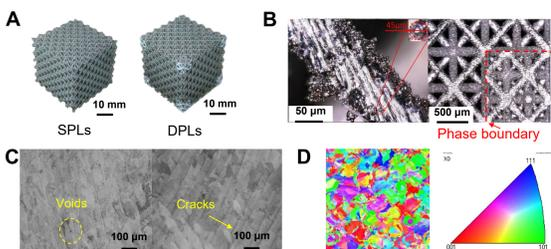
Fig. 2 (A) DPL samples fabricated by selected laser melting based additive manufacturing together with the single-phase counterparts. (B) Mesoscopic printing details. (C) Manufacturing defects observed. (D) EBSD characterization
