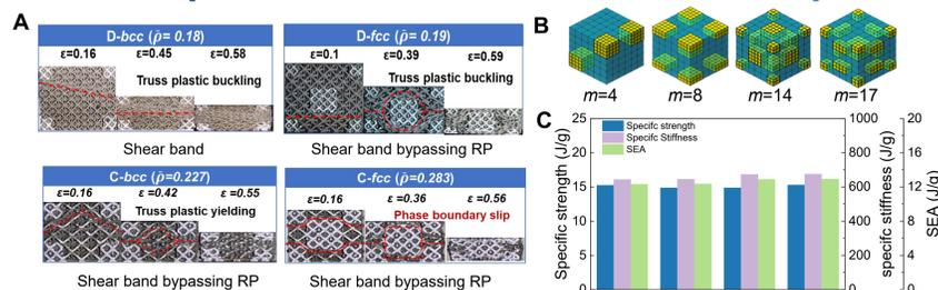
Fig. 4. (A) Typical deformation and failure modes illustrating localized shear bands in the different materials. (B-C) Stiffness, strength and energy absorption of DPLs with increasing complexity and reinforcement grain numbers  $m$  at constant volume fraction  $V_{RP}$ .
