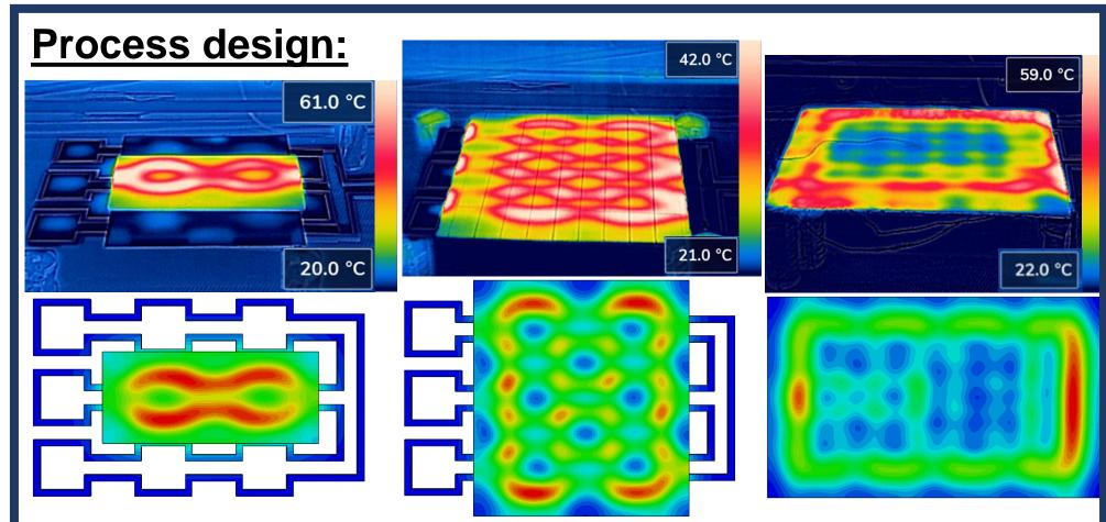
**Above:** (Top) Experimental temperature variation with different QI carbon fibre panel sizes. (Bottom) Modelling results for same sized panels.
