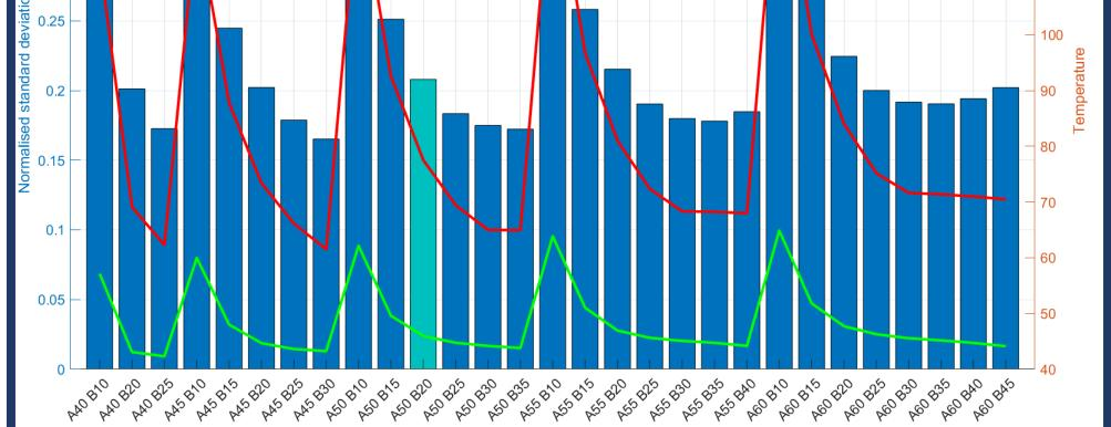
**Above:** Graph showing parametric design varying size and spacing of each cell. Focusing on reducing standard deviation to improve inplane temperature uniformity and maximising average temperature for heating efficiency. Light blue bar indicates current experimentally tested geometry.
