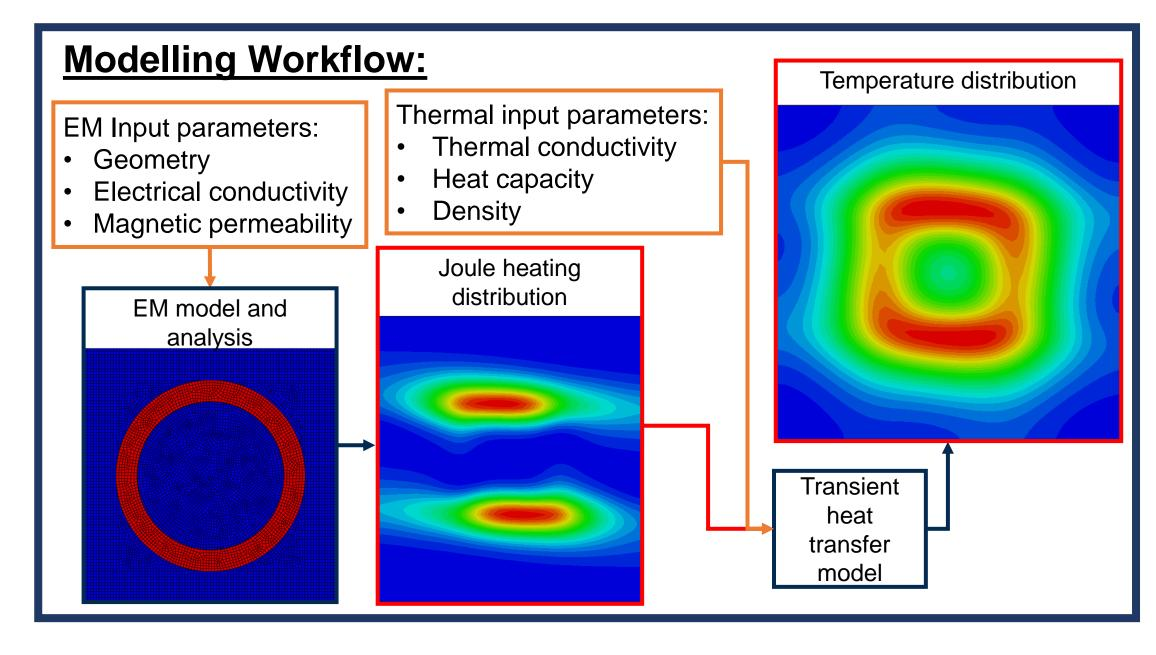
trialled. Each cell forms isolated EM vortices if the process parameters are properly tuned. Each EM vortices imprints a pattern of Eddy currents and Joule heating.
