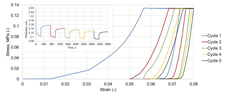
Stress –strain curves shows highly non-linear and visco-plastic behaviour. The area of the hysteresis loop initially decreases and then reaches the equilibrium
