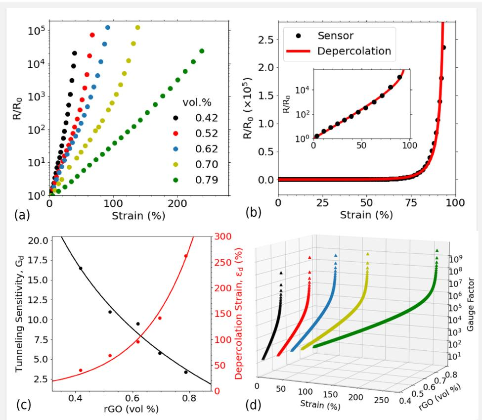
**Fig. 3.** Strain sensing. (a) Resistance variation of SR/rGO films under tensile strain. (b) Calibration using the depercolation model. (c) Depercolation model parameters for SR/rGO strain sensors. (d) Gauge factor of SR/rGO strain sensors as a function of strain, as predicted by the depercolation model.
