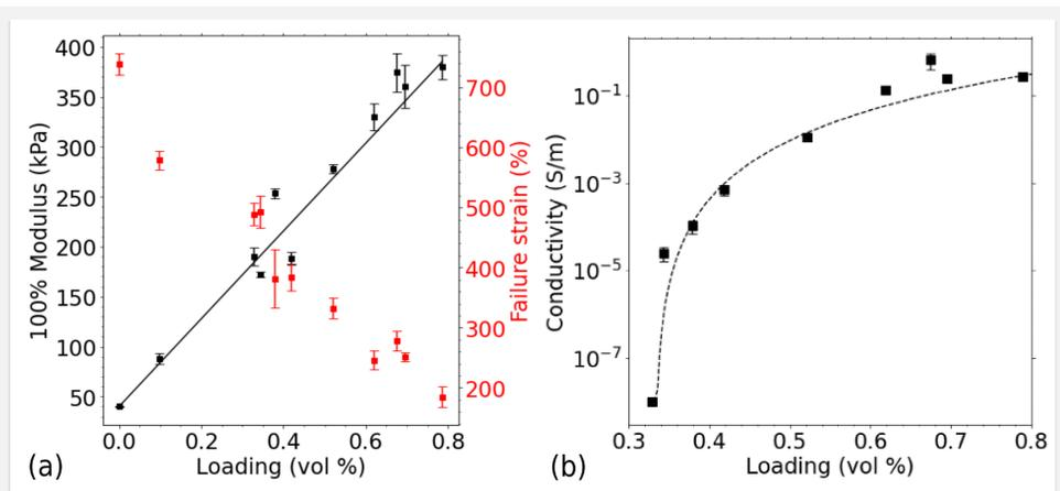
**Fig. 1.** SR/rGO nanocomposites. (a) 100% modulus (black) and strain at break (red). (b) Electrical conductivity displaying percolation at 0.33 vol %.
