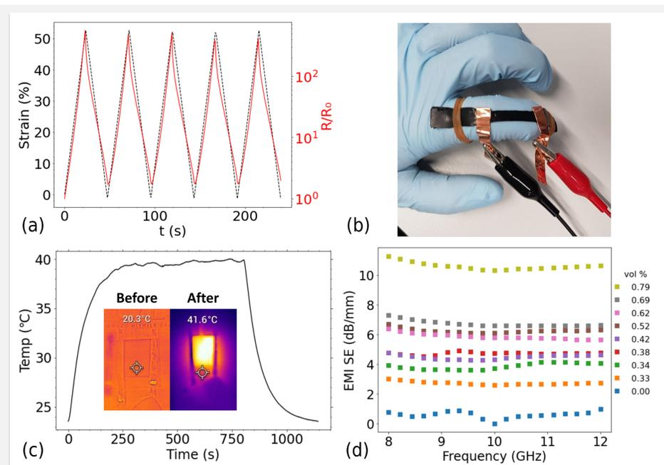
**Fig. 2.** Multifunctional properties. (a) Cyclic strain sensing. (b) Wearable strain sensor measuring repeated finger bending. (c) Joule heating at 10V. (d) EMI shielding.
