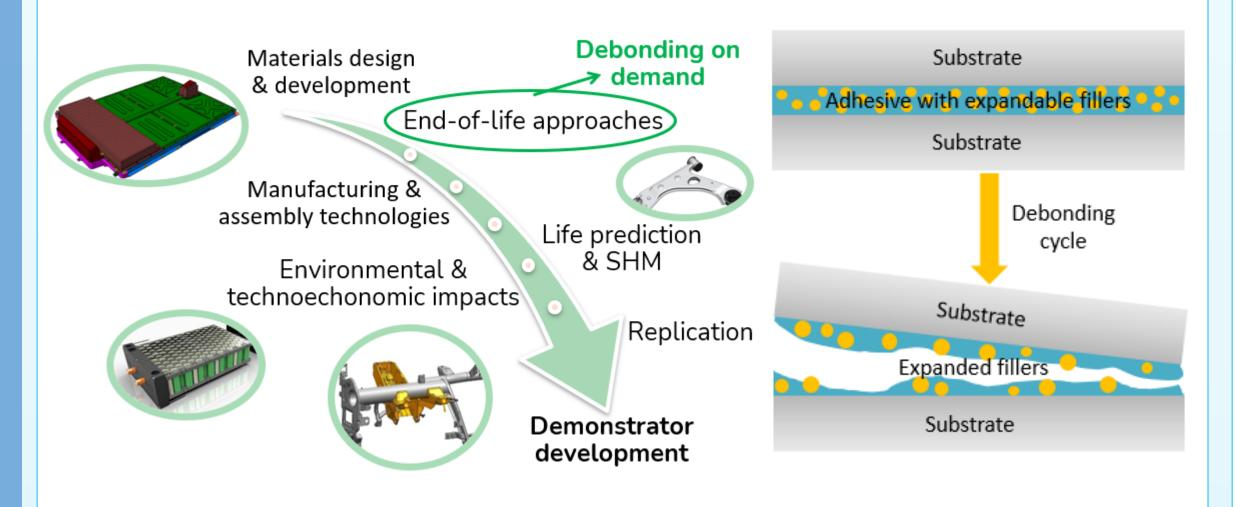
This work presents part of the investigation done about the introduction of TEPs/TEMs in a methacrylate adhesive (BOSTIK<sup>®</sup>) SAF 30/45), a commercial system selected to solve some specific hybrid metal-composite joints proposed in the project, to introduce the debonding on demand capability. Overall, high debonding effectiveness (%DE) was reached when a proper debonding cycle and concentration of particles are used.
