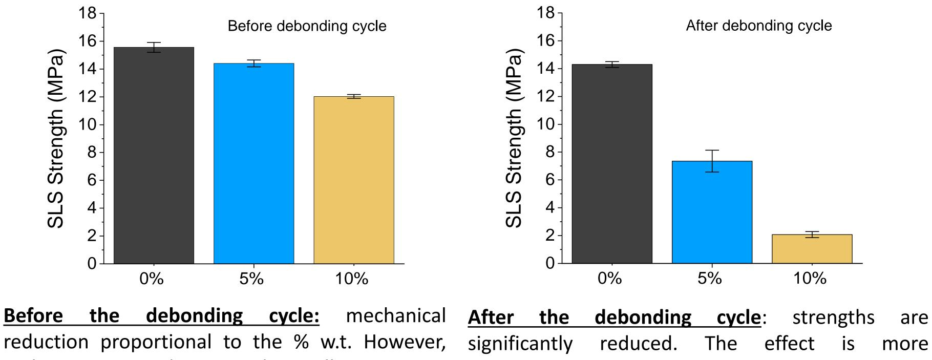
with a 10% w.t., the strength is still in a proper pronounced for the higher TEPs concentration. range for a structural adhesive for the LEVIS
