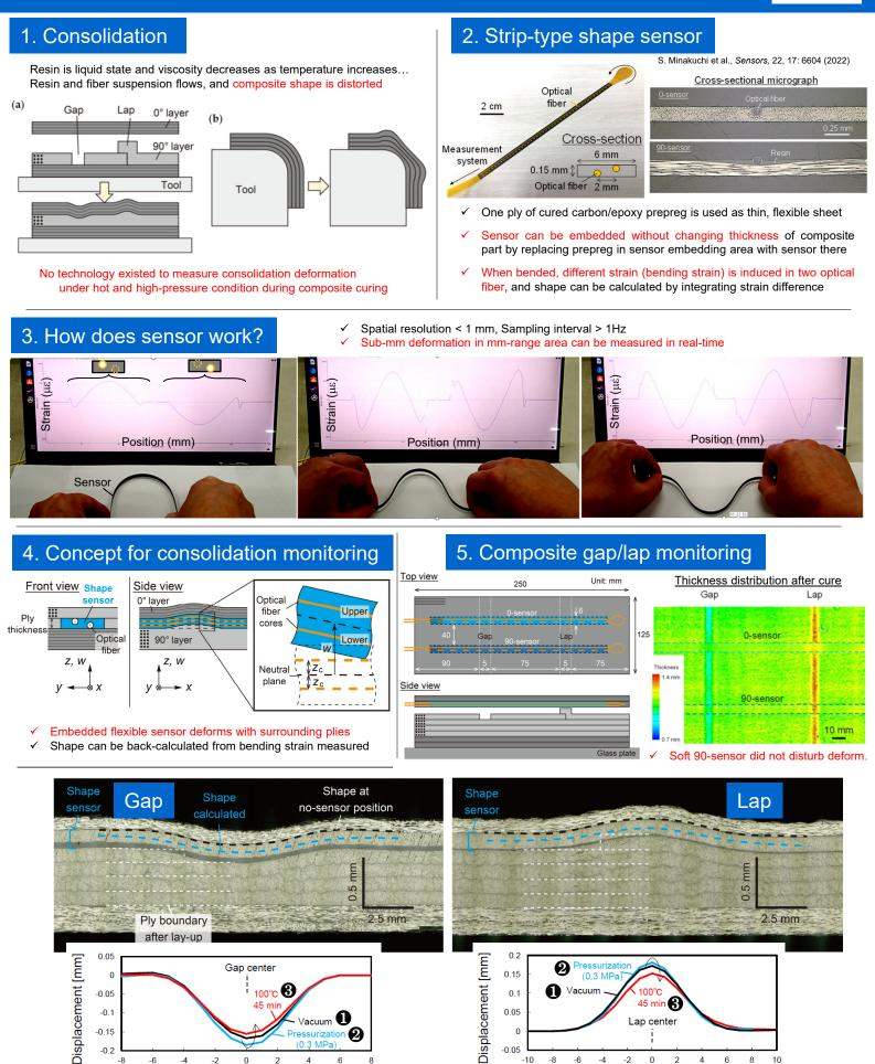
Shape calculated from sensor agreed well with cross-sectional observation ✓ Deformation deepened once and then became shallower as resin/fiber flowed
