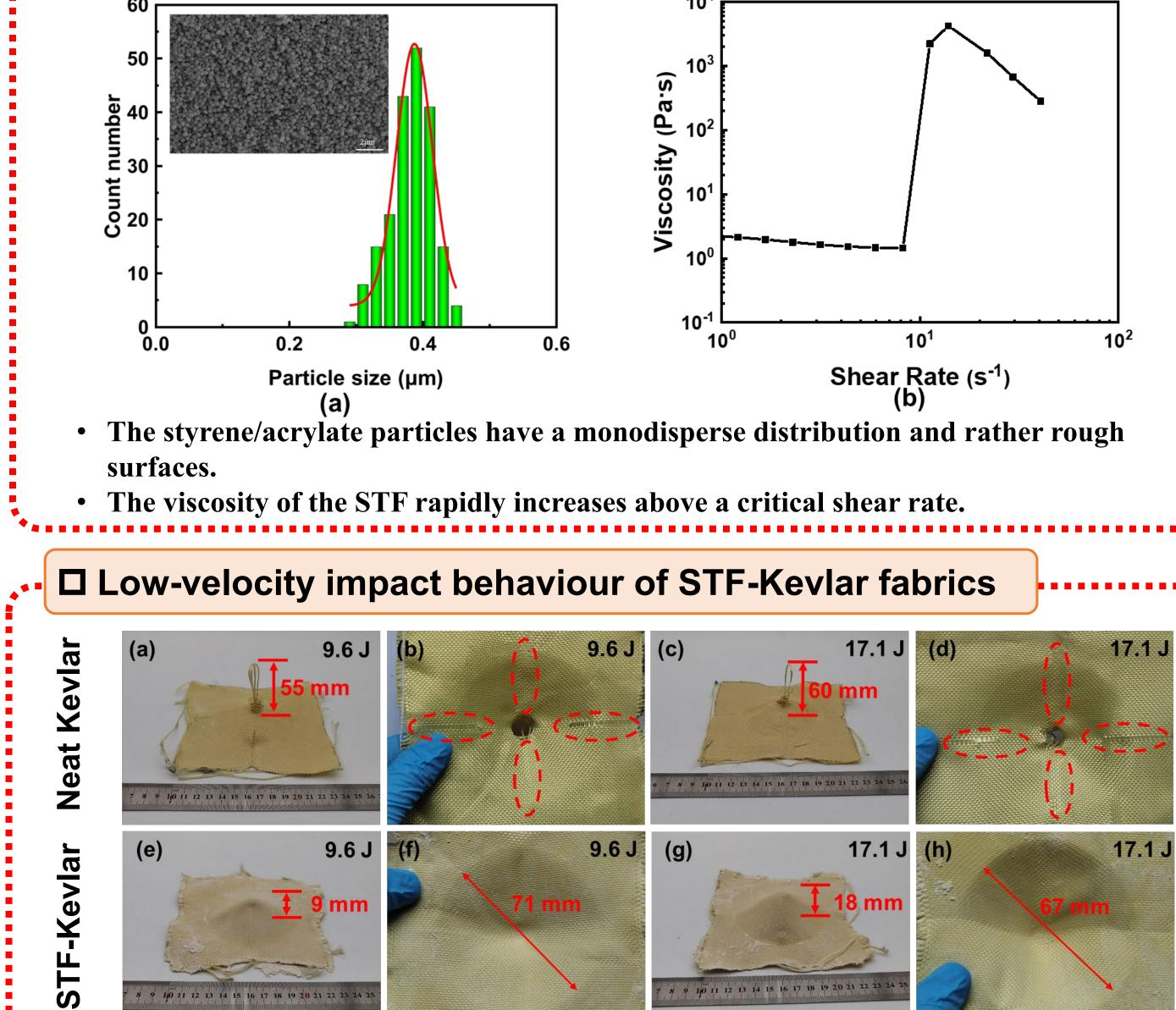
The addition of the STF and Kevlar fabrics greatly improves the impact resistance of ASP and decreases the maximum impact displacement.
