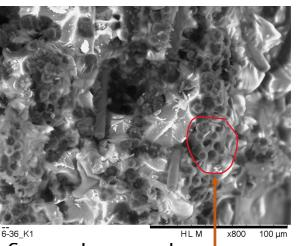
6mm – Improved Fibres oriented perpendicular to fracture surface
