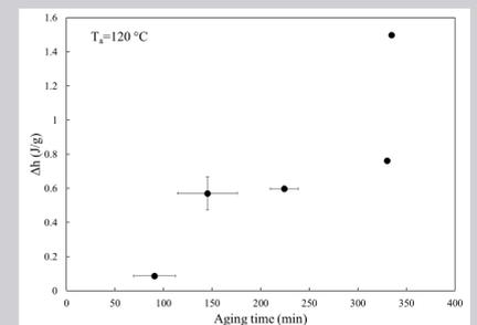
Fig. 8 evolution of the enthalpy of aging as a function of aging time for 8552 resin held at 120 °C for different aging times
