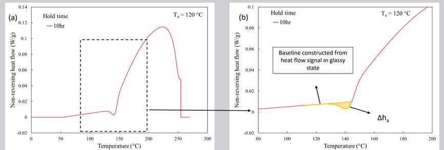
Fig. 6 (a) heat flow signal of 8552 resin after 10 hours at 120 °C, during the heating step to 270 °C at 2 °C/min (b) zoomed view of fig. 6(a); the area under the curve of the endothermic peak represents enthalpy of aging.
