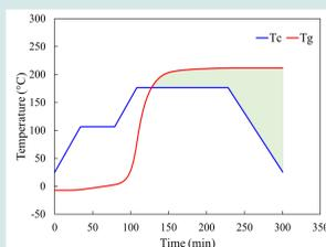
Fig.2 Manufacturer recommended cure cycle (MRCC) for Hexcel 8552 resin. Glass transition temperature ( $T_g$ ) exceeds cure temperature ( $T_c$ ).
