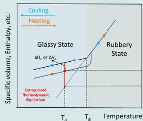
Fig.1 evolution of thermodynamic properties due to physical aging at the aging temperature of  $T_a$
