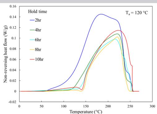
Fig.4 DSC heat flow signal during the heating step to 270 °C at 2 °C/min, following the isothermal hold at 120 °C. Hold times vary between 2 to 10 hours.
