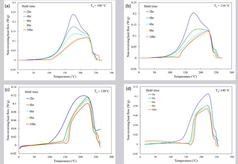
Fig.5 DSC heat flow signal during the heating step to 270 °C at 2 °C/min following an isothermal hold at (a) 100 °C, (b) 110 °C, (c) 130 °C, and (d) 150 °C. Hold times vary between 2 to 10 hours.
