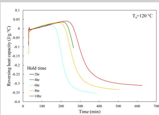
Fig.3 Reversing component of heat capacity of 8552 resin during an isothermal hold at 120 °C for different hold times
