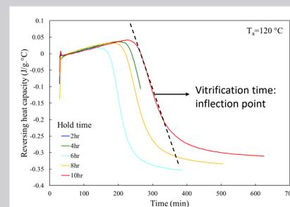
Fig. 7 true aging times are calculated using the inflection point of the heat capacity step change
