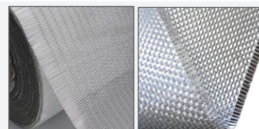
Unidirectional glass-fiber (UD-GF) 640 g/m 2 0/90° Bidirectional glass-fiber (BD-GF) 580 g/m 2 0/90°
