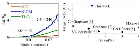
Sensitivity,  $GF = (\Delta R/R_0)/\epsilon$ , increased due to changes in contact resistance resulting from two factors:
