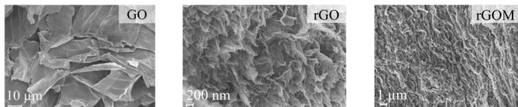
The porous structure was produced by phase separation between water and rGO networks, which occurred as a result of L-cysteine reduction in the GO suspension.
