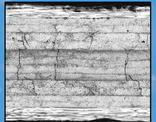
Typical Image of Microcracks in Composite Specimens, Layup  $[90_2/45_2/-45_2/0_2]_s$
