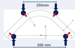
FIGURE 6. LOADING GEOMETRY
