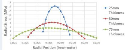
FIGURE 2. EFFECT OF THICKNESS ON RADIAL STRESS DISTRIBUTION THROUGH THICKNESS
