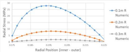
FIGURE 3. EFFECT OF CURVATURE ON RADIAL STRESS DISTRIBUTION THROUGH THICKNESS
