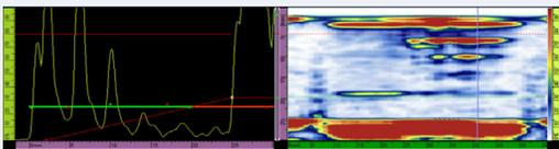
FIGURE 8. TYPICAL ULTRASOUND RESULTS (LEFT: ASCAN, RIGHT B-SCAN)
