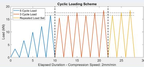
FIGURE 7. CYCLIC LOADING SEQUENCE
