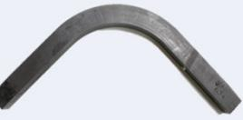
FIGURE 5. FULL THICKNESS CURVED COMPOSITE SPECIMEN
