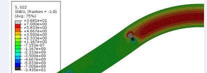
FIGURE 4. THROUGH THICKNESS STRESS DISTRIBUTION
