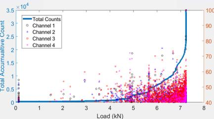
FIGURE 10. DAMAGE EVOLUTION FOR 25MM THICK RS1
