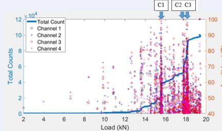
FIGURE 9. DAMAGE EVOLUTION FOR 40MM THICK RF1
