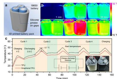
Fig.5 (a) Battery test setup. (b) IR images of pure TPU pack (left) and Gr/TPU pack (right). (c) temperature
