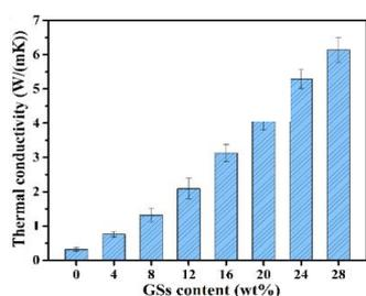
Fig.1  $TC^\perp$  of Gr/PA6 composites
