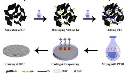
Fig.2 Schematic for the fabrication of NUL-Gr/CFs and NUL-Gr/CFs/PVDF composite
