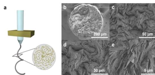
Fig.3 (a) Schematic of extruded micro-filament. (b) Morphology of micro-filament (c-e).
