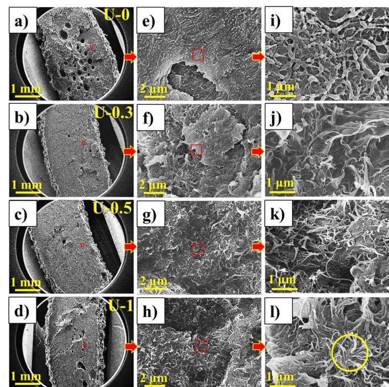
**Fig. 5** SEM images of fracture surfaces corresponding to 3D printed pure UHMWPE (top row) and MWCNT/UHMWPE nanocomposites (bottom and middle rows); the circle in (l) shows agglomerates of MWCNTs.
