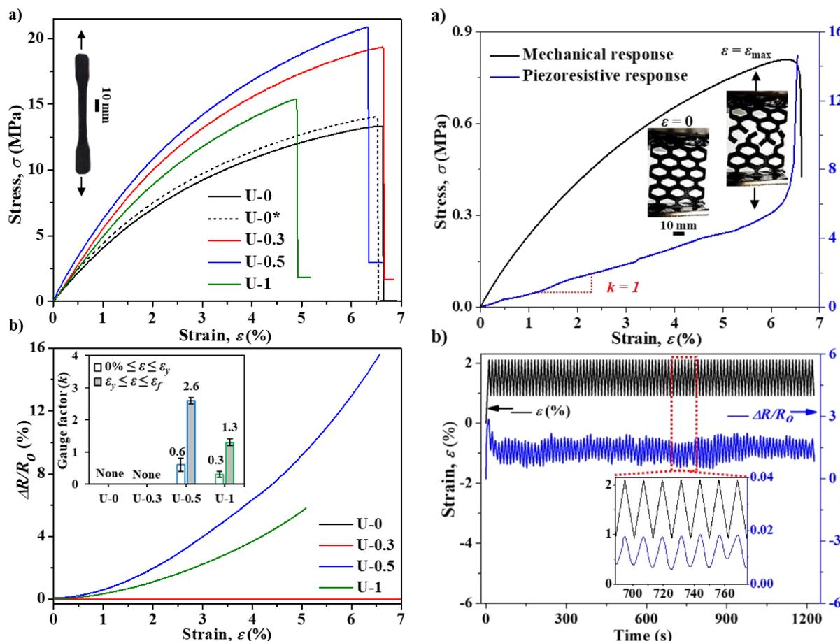
**Fig. 2** Mechanical and piezoresistive behavior of MWCNT/UHMWPE nanocomposites under uniaxial tension: (a) stress-strain response (b) piezoresistive response. Inset in (b) shows gauge factors calculated in elastic and inelastic regimes. Note: U represents the polymer matrix whereas numerals (0.3, 0.5, 1) are wt.% of MWCNT. U\* represents the ballmilled pure polymer.  $\epsilon_y$  is yield strain and  $\epsilon_f$  is fracture strain.
