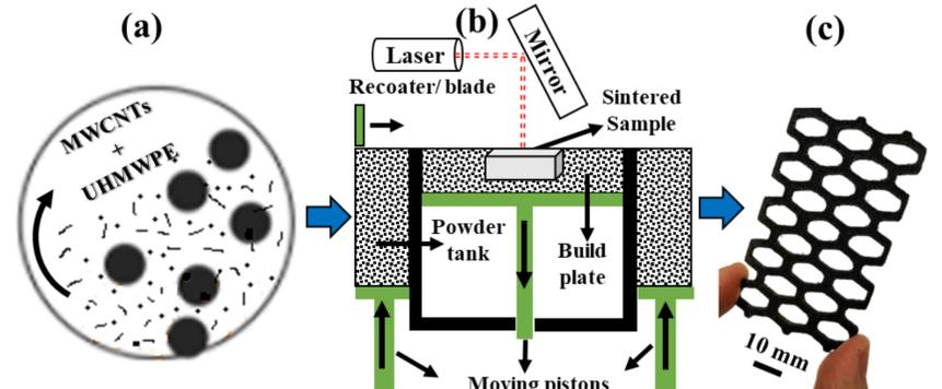
**Fig.1** Schematic of steps involved in processing of MWCNT/UHMWPE nanocomposites via SLS: (a) preparation of nanocomposite powders via ball milling, (b) 3D printing via SLS, (c) 3D printed structure.
