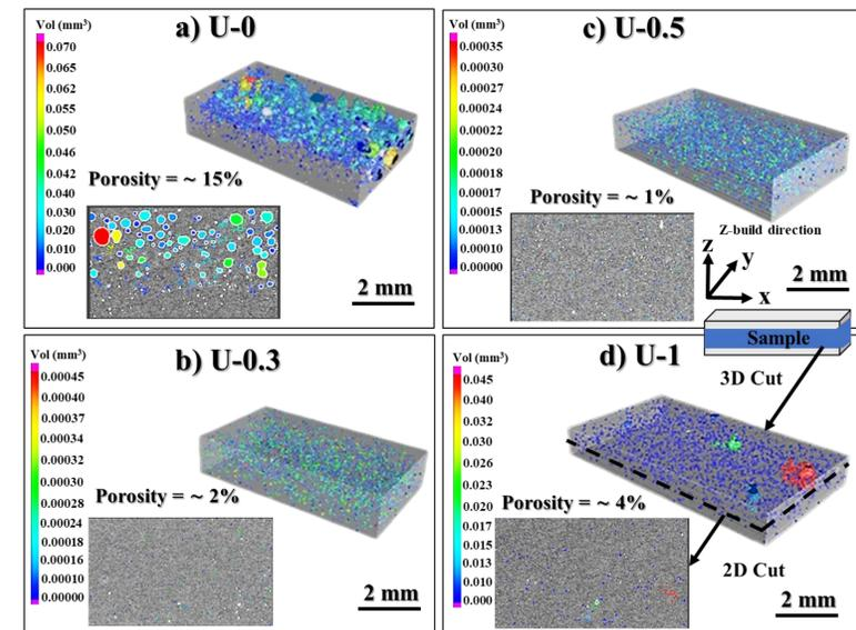
**Fig. 4**  $\mu$ CT analysis of (a) pure UHMWPE (b-d) MWCNT/UHMWPE nanocomposites.
