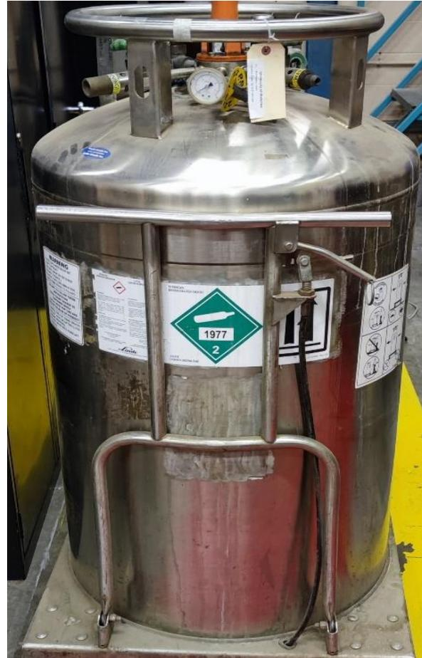
*LN2 canister used to cool climate chamber for LT tests.*
