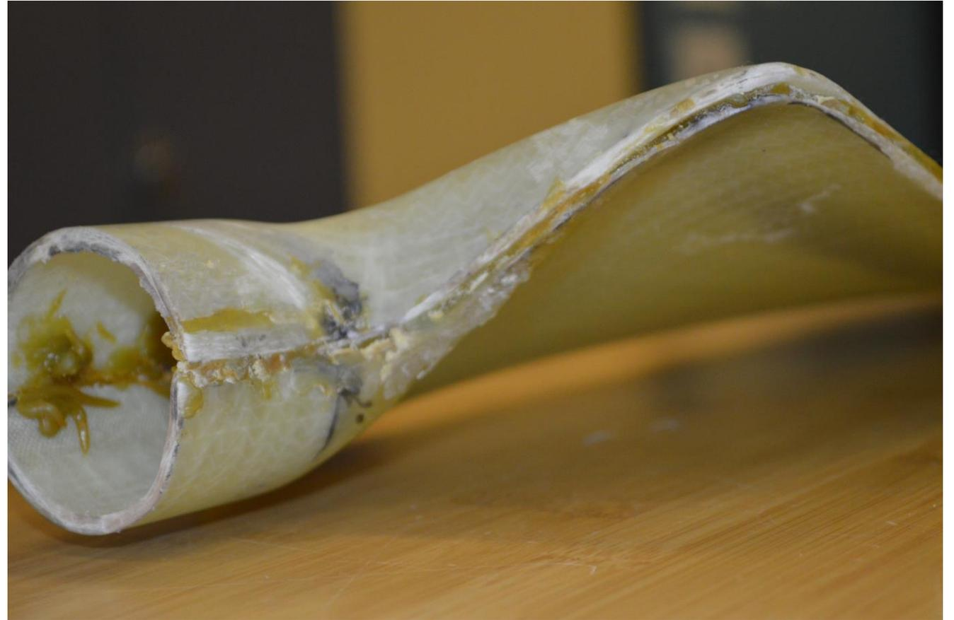
*Adhesive-bonded micro-generating wind turbine blade.*
