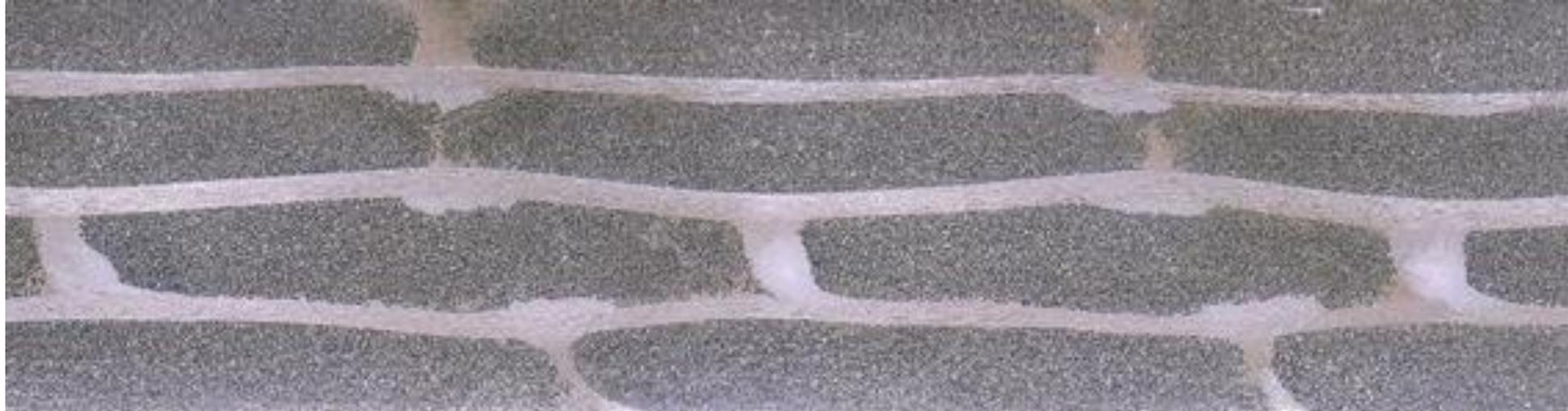
*Cross-sectional image of thermoplastic fiberglass panel.  $[0]_4$  stacking sequence with  $\approx 48\%$  FVF.*
