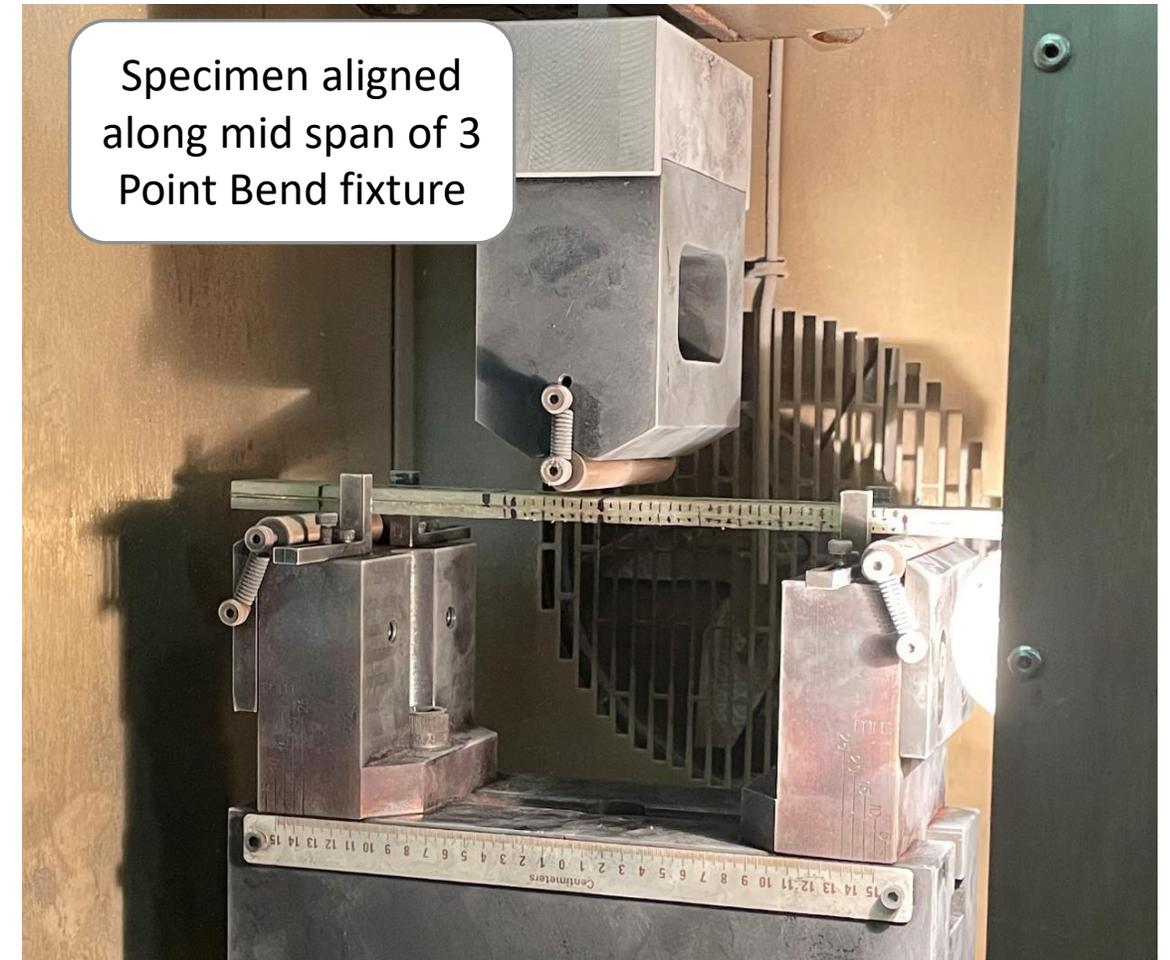
*3 Point Bend (3PB) fixture setup for ENF testing.*
