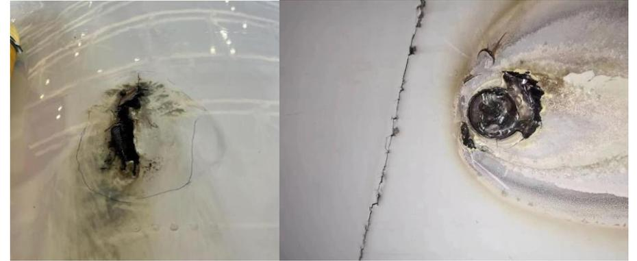
Damage on aircraft by lightning strike
