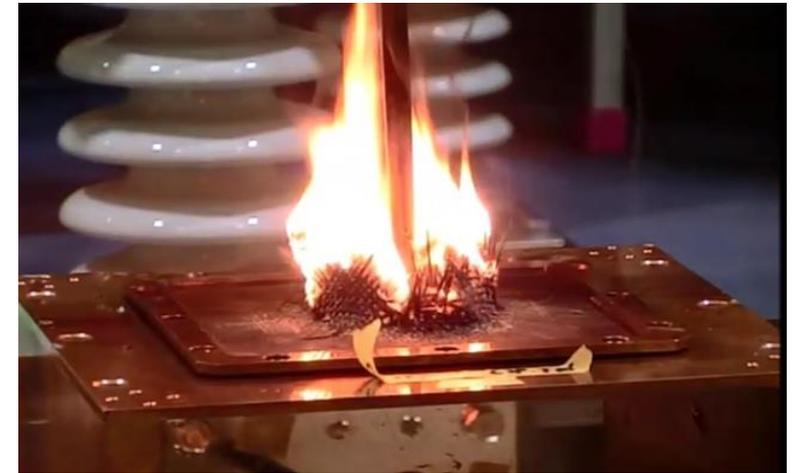
CF/Epoxy laminate strike by simulated lightning
