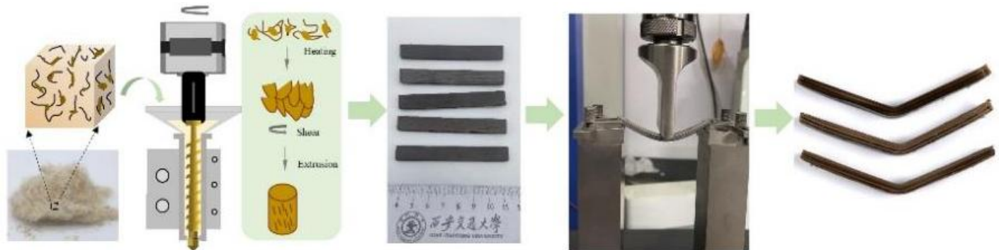
Sketch of recycle PPS CFSRCs screw extrusion 3D printing process
