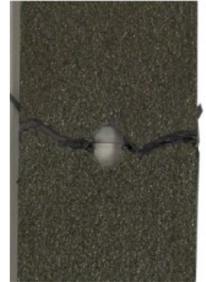
Hard Composite in Tension
