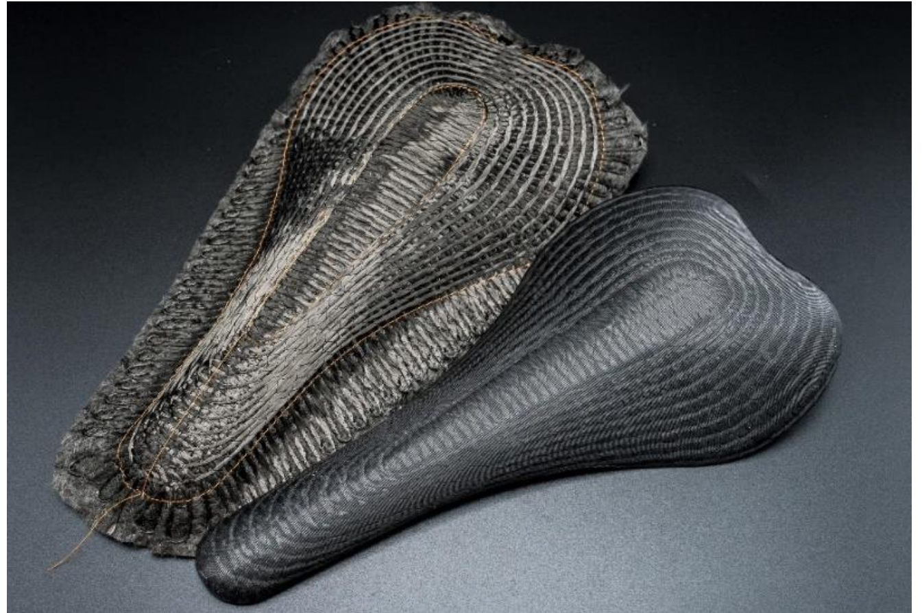
Demonstration part “bike saddle”: TFP-CF on rCF nonwoven preform (top) and consolidated part (bottom), rCF content > 50 %, Embroidery pattern created with EDOpath
