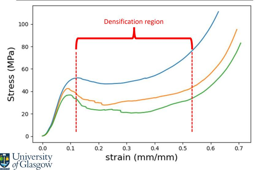
• Achieved the successful reinforcement of mechanical properties by the coating and increase of up to ~10 fold energy absorption due to smooth densification region in failure mechanism in cellular material.
