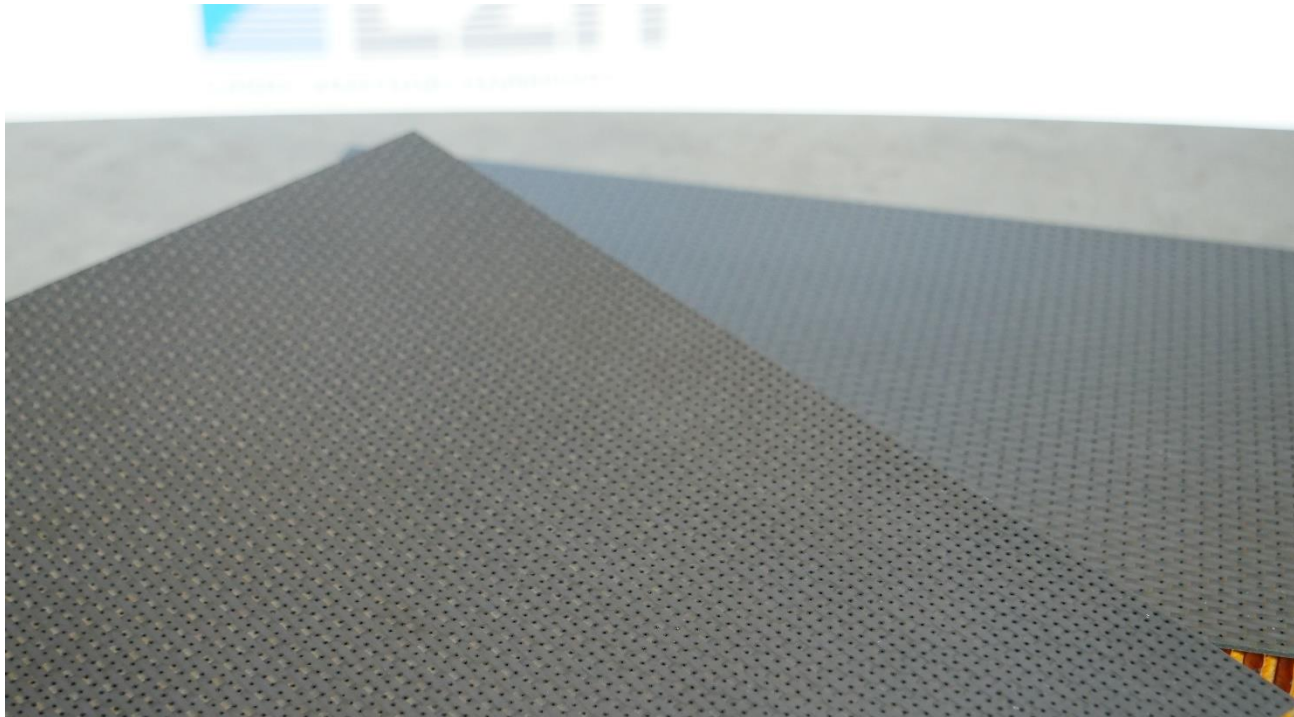
Laser-machined carbon fiber-reinforced honeycomb panel with microbores
