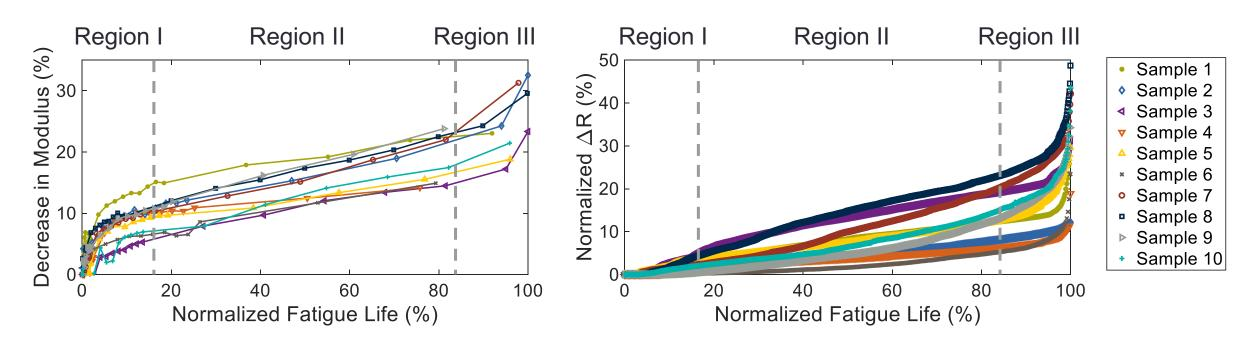
Region I: dominant form of damage is matrix cracking especially within off-axis plies
