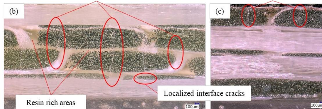
Microscopic observation of RT samples: (a) axial direction at 20%UTS,
