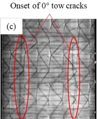
Onset of  $0^\circ$  tow cracks
