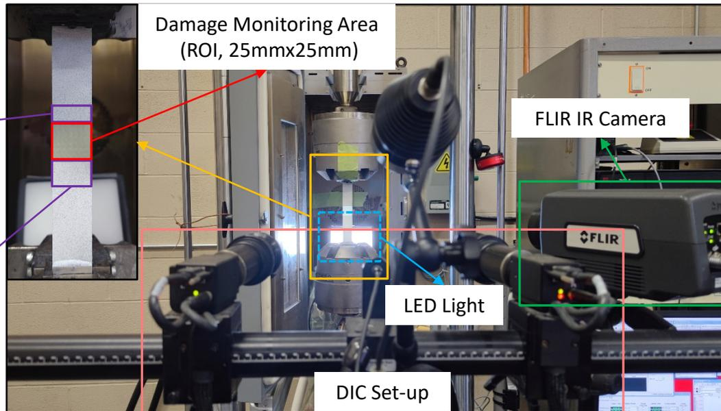
Test set-up for fatigue test
