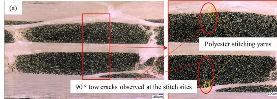
Cracks coalescence between the  $90^\circ$  fiber layers
