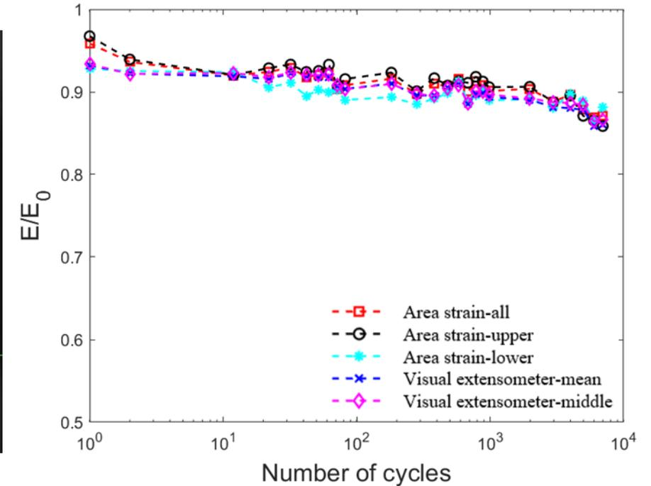
Stiffness degradation at room temperature (50% UTS)
