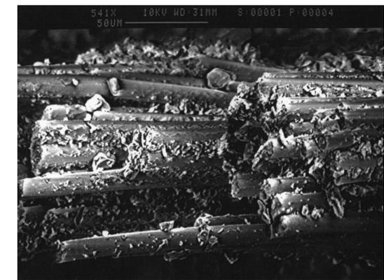
Brittle failure mode of FRP composites at low temperature
