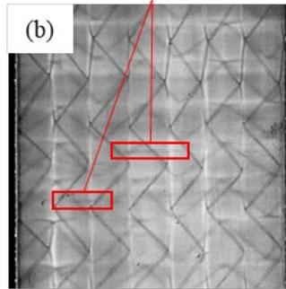
Examples of  $90^\circ$  ply fiber towDevelopment of  $90^\circ$  tow cracks
