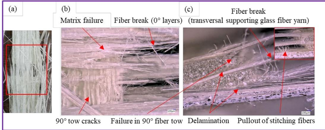
RT test specimen: (a) image of front fracture surface, (b) photomicrographs of front fracture surface, (c) photomicrographs of side fracture surface.
