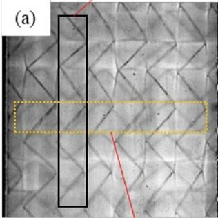
Onset of  $90^\circ$  tow cracks
