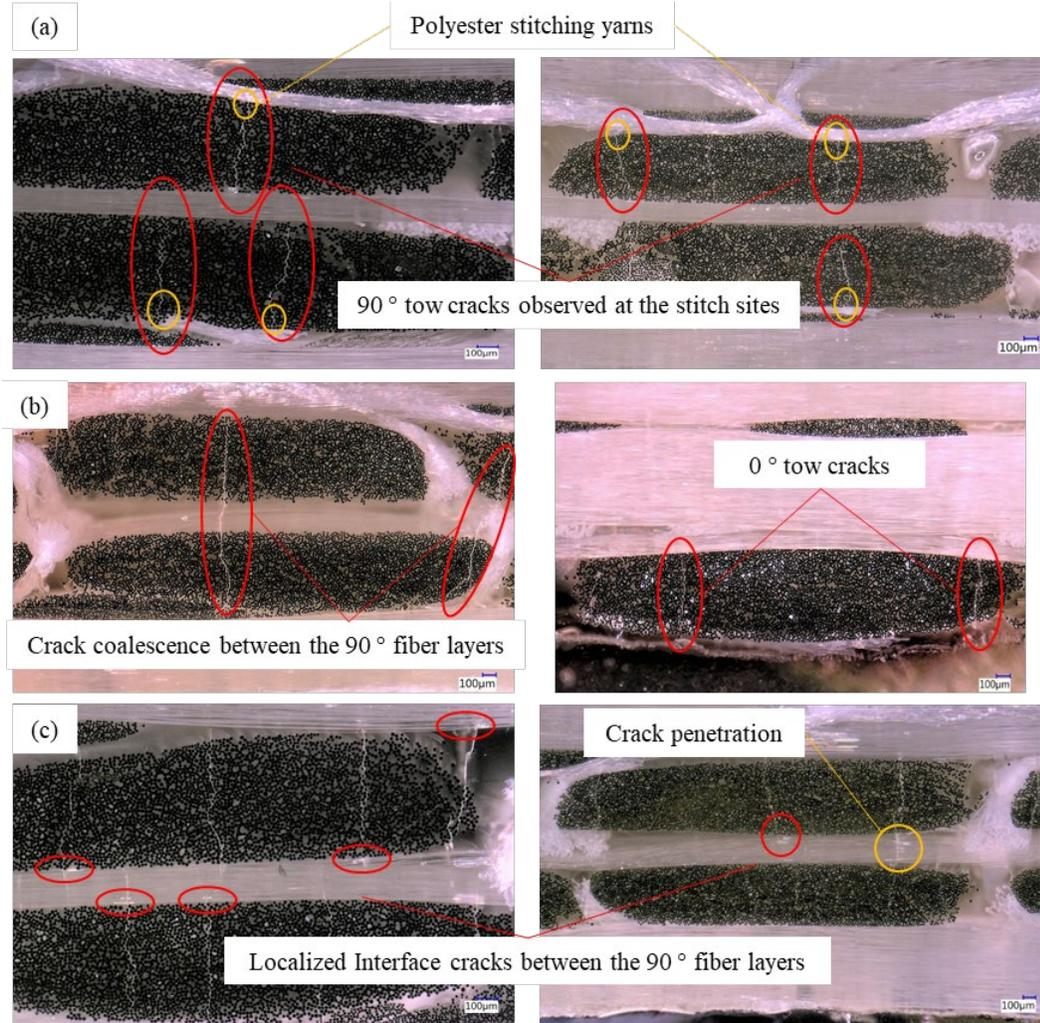
Microscopic observation of  $-50^\circ\text{C}$  samples (a) axial direction at 20% UTS, (b) axial and cross-section direction at 50% UTS, (c) axial direction at 70%-75%UTS.
