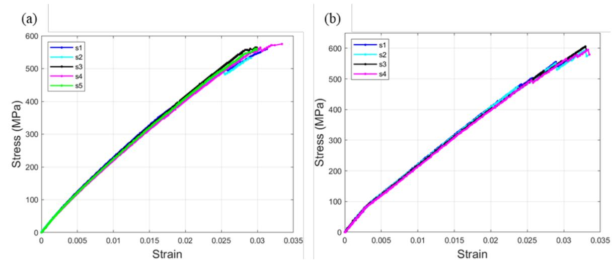
Laminate stress-strain response (a) RT, (b) -50°C
