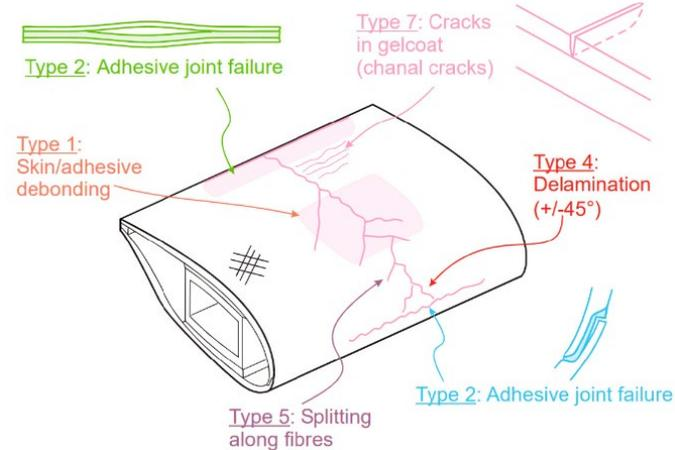
Typical failure modes of wind turbine blades [2]
