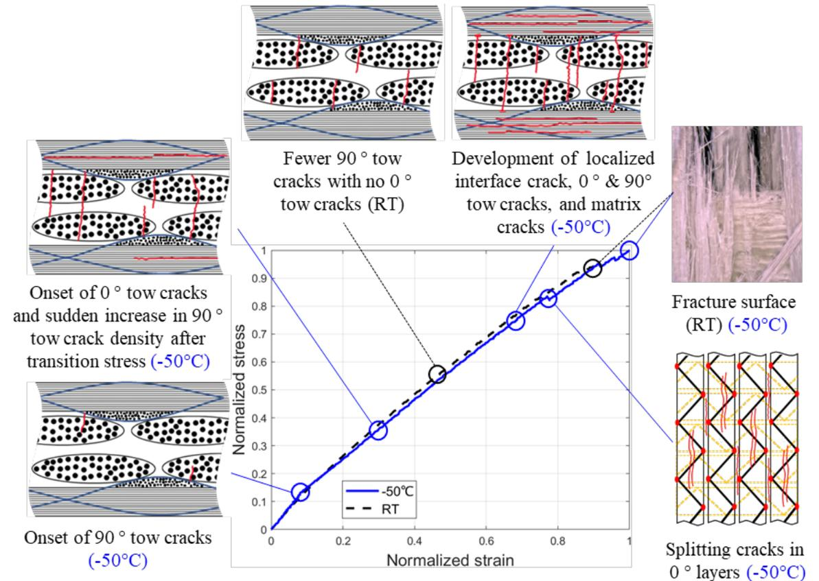
Schematic of damage evolution during static loading (only resin rich area between 90° fiber layers was shown)
