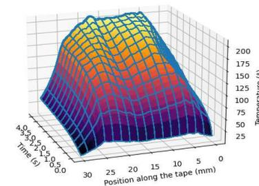
Temperature measurement on a metallic target, with a gaussian profile for intensity (request for more energy on the center and less on the edges).
