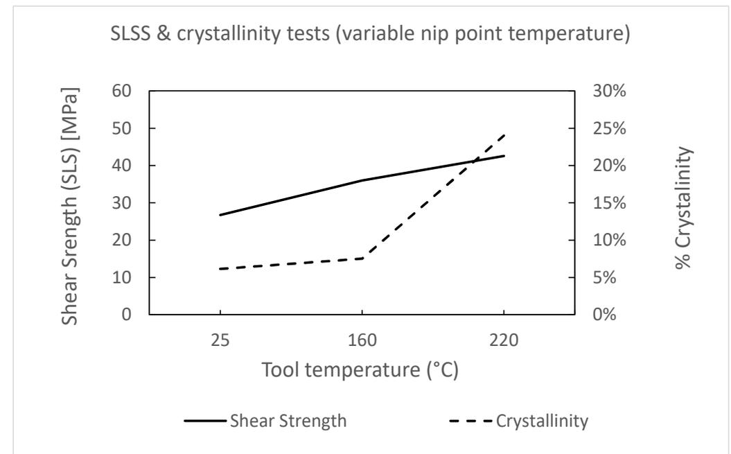
Higher substrate temperature higher crystallinity and higher SLSS
