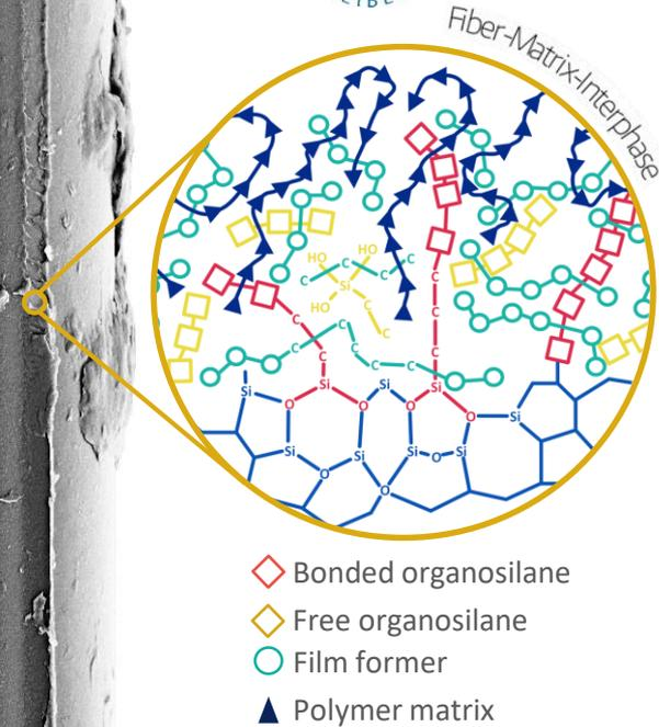
**My aim:** development and analysis of a suitable biodegradable and biobased sizing for degradable glass fibers
