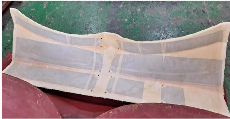
(d) 1:1 scale heating panel specimen production completed
