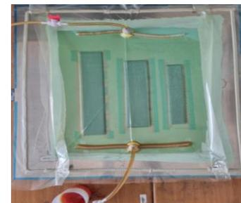
(e) Curing and demolding
