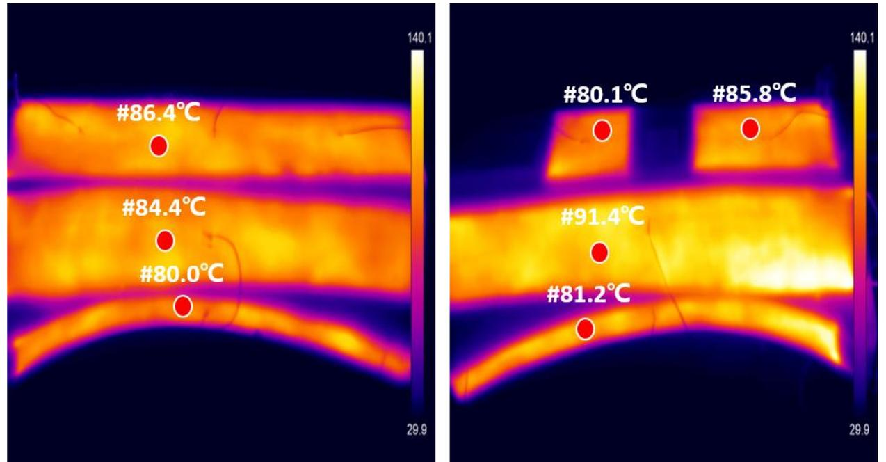
Infrared thermal image of self-heating composite panel
