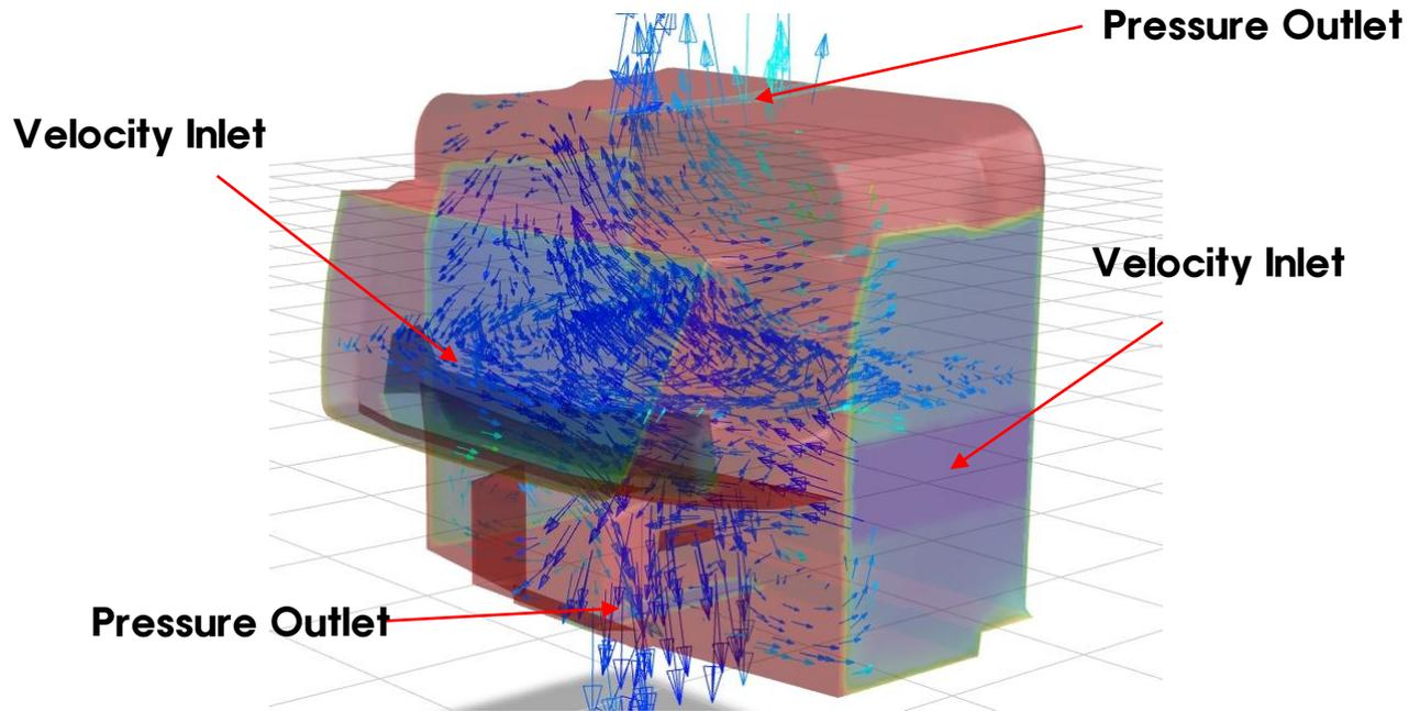
Example of air flow inside the cab
