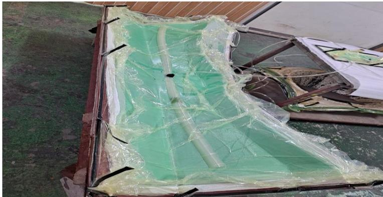
(c) Vacuum pressure and injecting resin
