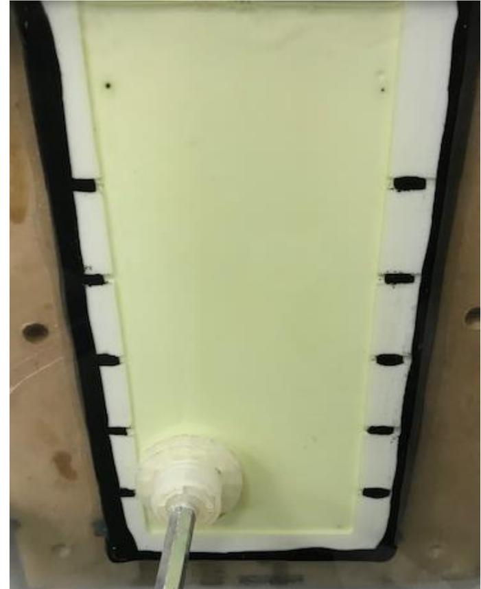
Sealed fragmentation mould with resin and fibres
