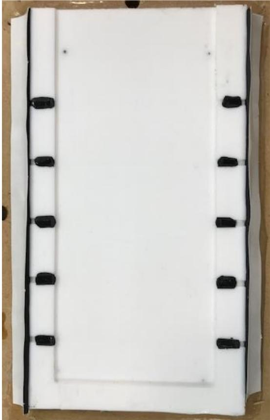
Fragmentation mould prior to sealing and addition of resin
