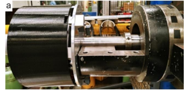
Mounting the platform and the drill tube on the drill chuck
