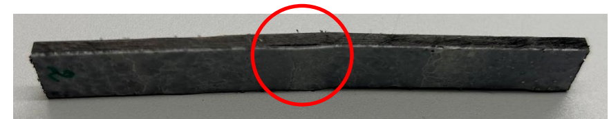
PA6/CF/3P%HPCTP/4%EGES100 sample after three-point bending test
