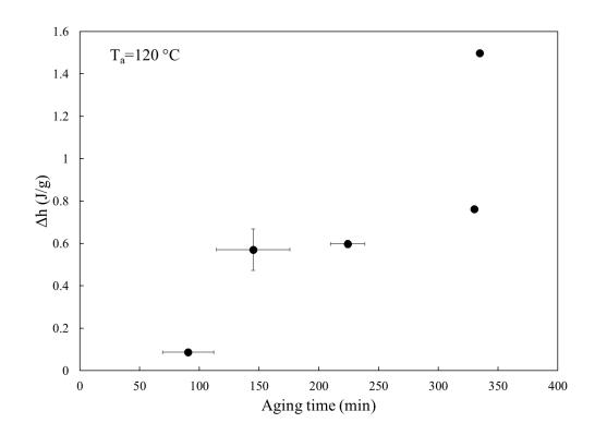
the aging enthalpy is seen to measurably increase over timescales relevant to composites processing.
