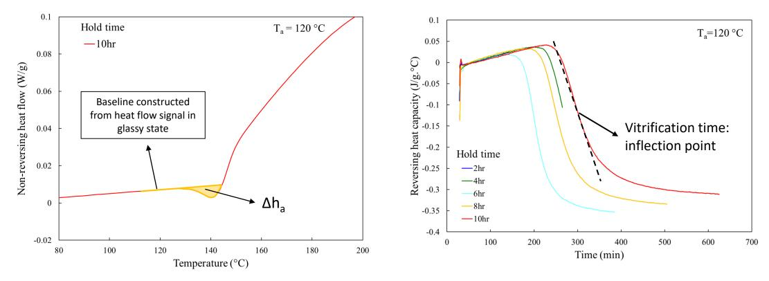
The baseline is constructed as a tangent line to the heat flow signal of the DSC test in the glassy range.
