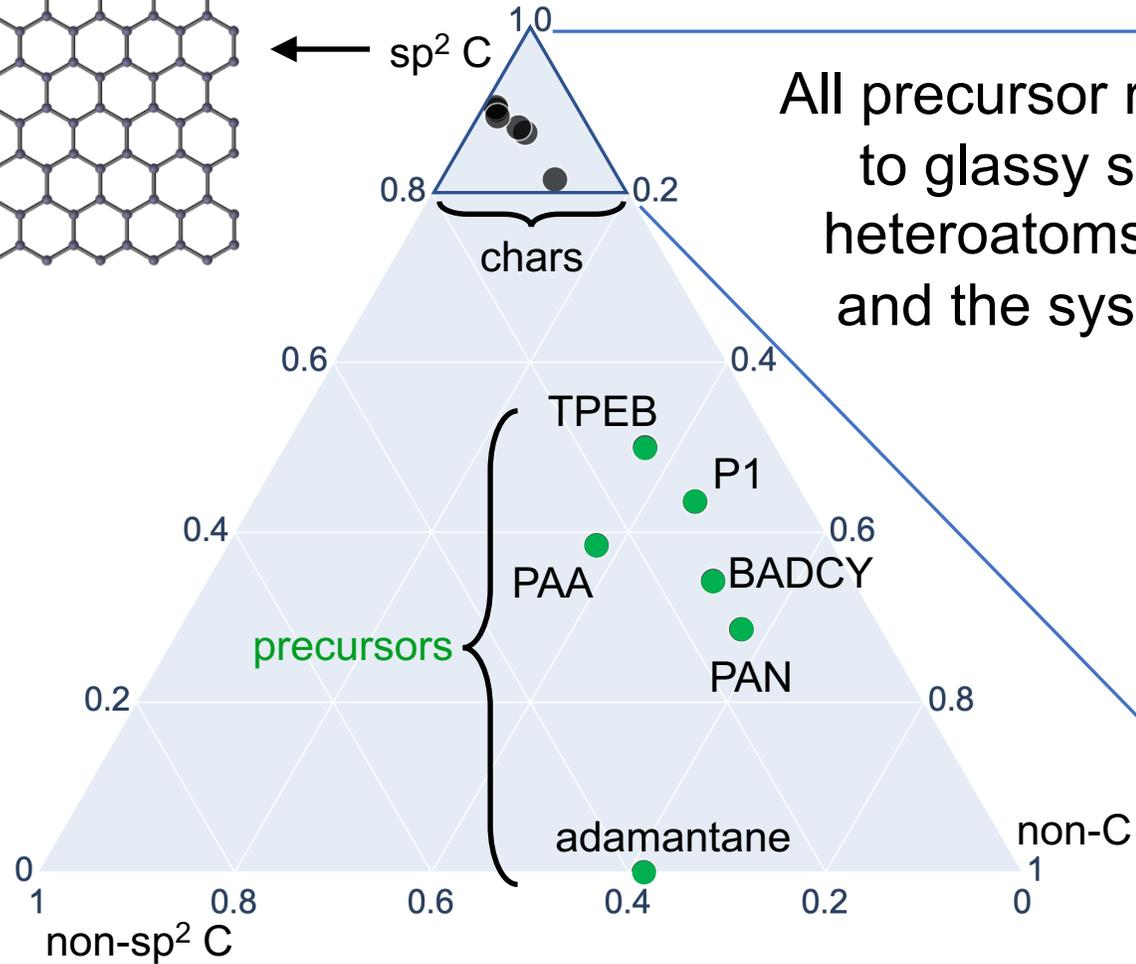
All precursor resins converge to glassy sp<sup>2</sup> carbon as heteroatoms are removed and the system densifies
