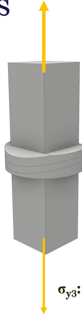
**σ<sub>y3</sub>: ASTM C297**
