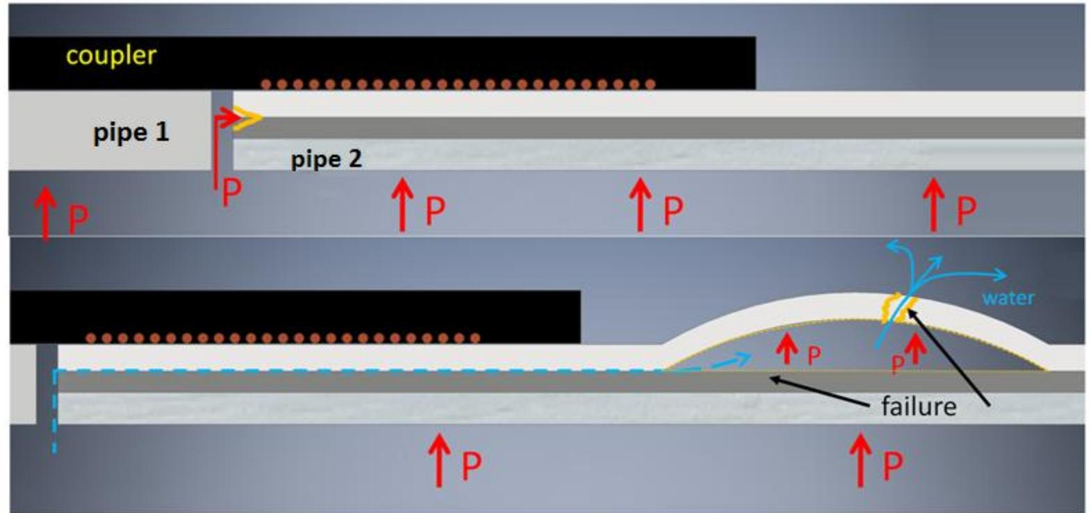
Conclusion: the dedicated coupler must isolate the reinforcement from the fluid!
