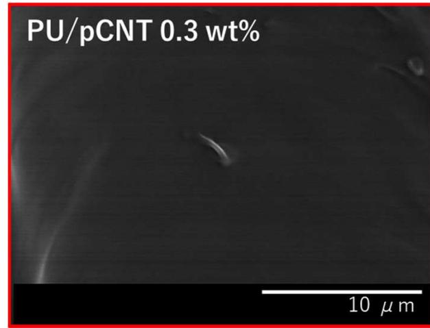
Figure. SEM images of PU and PU/CNT composite materials
