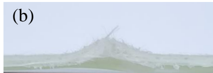
Side view of composite laminates after 30 J LVI loading, (a) [G^{40}]_2 , (b) [G^{60}]_2 , (c) [G^{40}/M/G^{40}]
