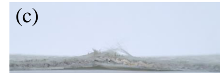
Side view of composite laminates after 30 J LVI loading, (a) [G^{40}]_2 , (b) [G^{60}]_2 , (c) [G^{40}/M/G^{40}]
