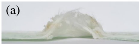
Side view of composite laminates after 30 J LVI loading, (a) [G^{40}]_2 , (b) [G^{60}]_2 , (c) [G^{40}/M/G^{40}]
