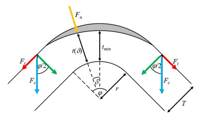
geometry parameters:  $\varphi$ , r, T (and L)
