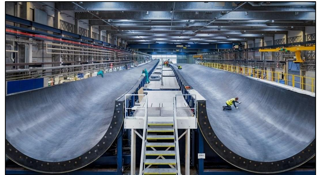
Heated mold for manufacturing a wind blade
