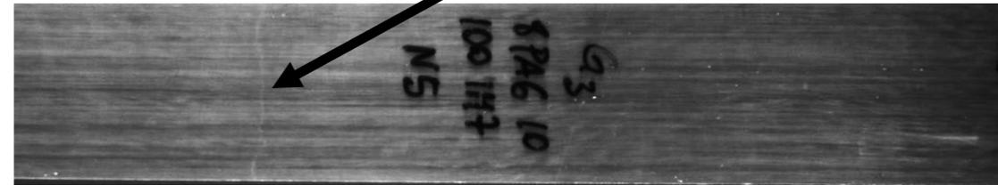
First fracture of the CF/EP layer
