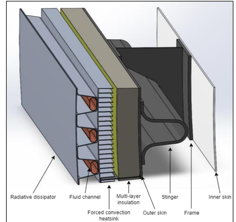
*Heat sink concept by radiation and forced convection*
