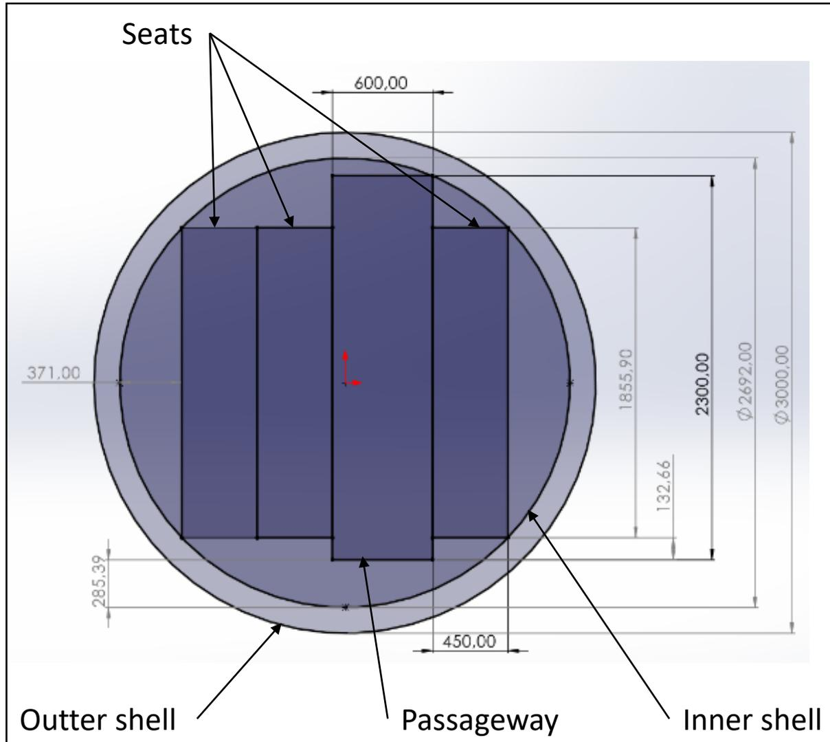
The interior dimensions are bus-like and maximized for a fixed hull diameter.
