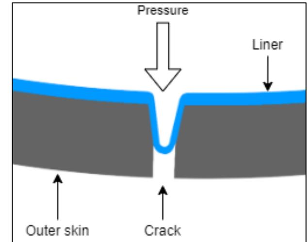
Schematic of self-sealing
