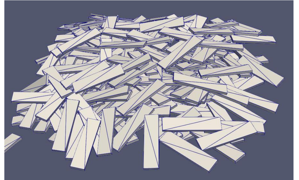
270 chips on a 150 mm * 150 mm deposition square Size of chips : 10 mm * 40 mm * 2 mm
