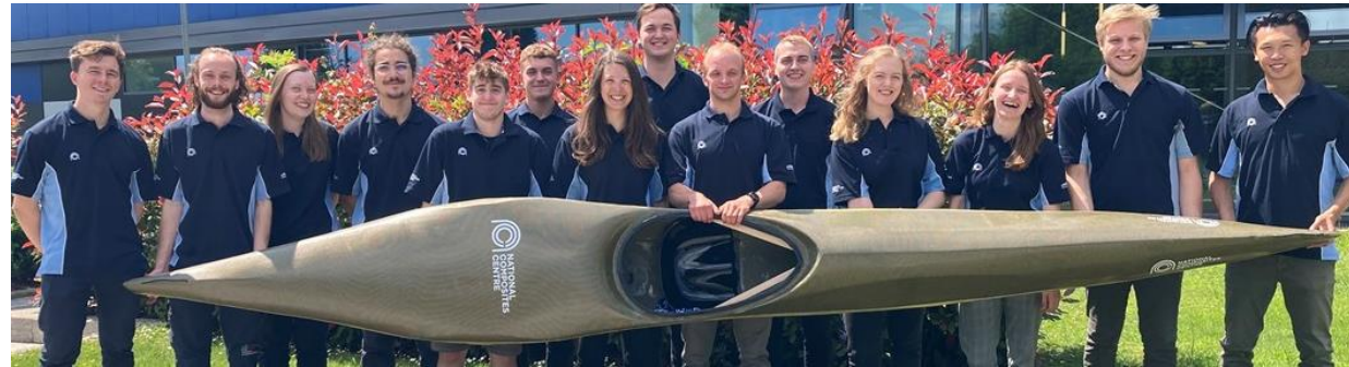
AFRP (Kevlar-49)/CFRP hybrid (infusion) Racing kayak Bisphenol A–derived epoxy with a design for degradation hardener, Recyclamine by Aditya Birla
