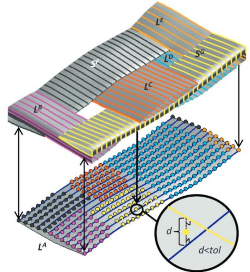
**Fig. 3.** Detection of contact zones between yarns. (For interpretation of the references to color in this figure legend, the reader is referred to the web version of this article.)
