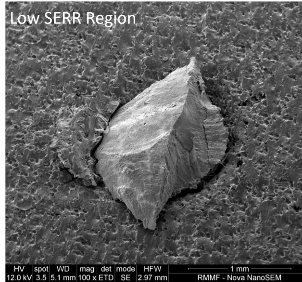
Figure 28. Ti-pin embedded in CFRP laminate; low SERR region
