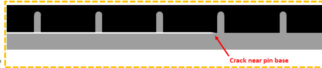
Figure 35. Mode I fatigue fracture at pin row
