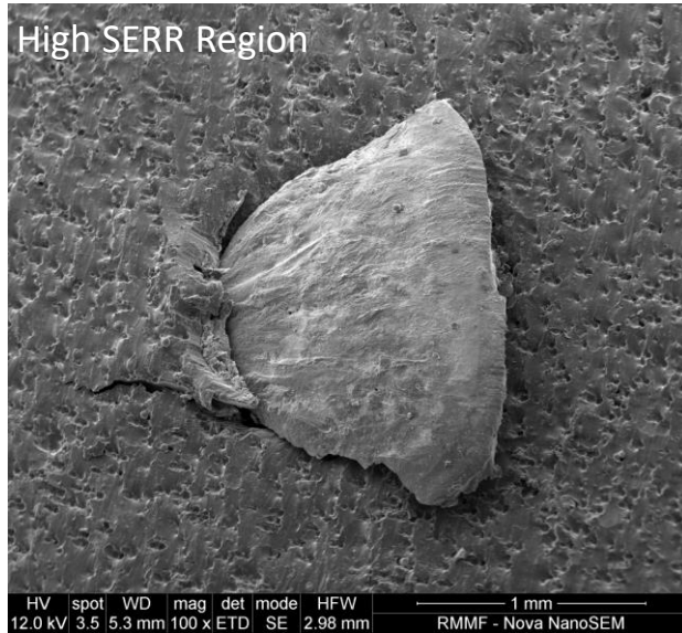
Figure 27. Ti-pin embedded in CFRP laminate; high SERR region
