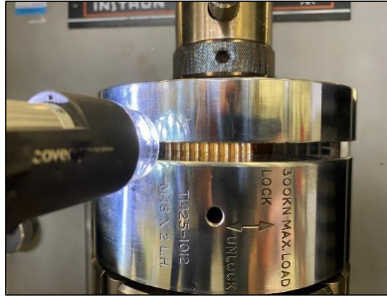
Figure 5: The setup of ASTM C365 (flatwise compression) experiment
