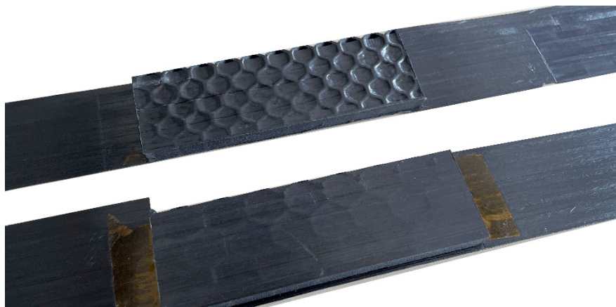
Figure 4: tapes laid onto 3d printed honeycomb structure with 100 % (upper) and 50% (lower) consolidation force
