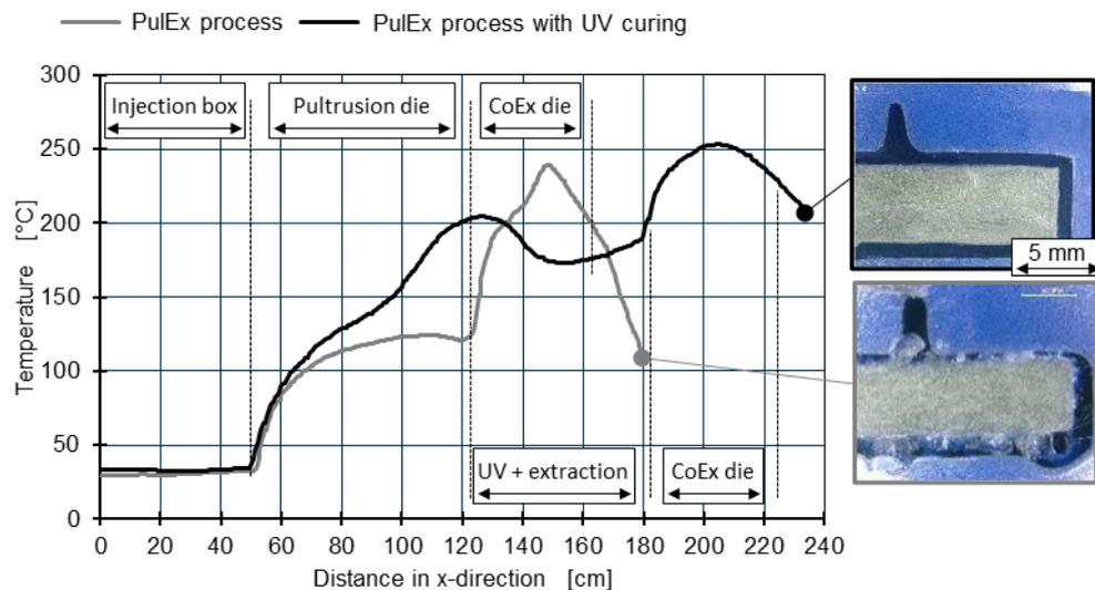
Figure 2: Temperature profiles in the center of the pultrusion profile for the PulEx process with ( $v_{pull} = 0.5$  m/min) and without ( $v_{pull} = 0.25$  m/min) dual curing. Cross-section of the PulEx profiles.
