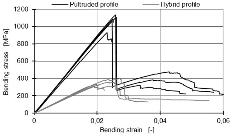
Figure 7: Stress-strain curve of pultruded and hybrid profile in a three-point bending flexural test.
