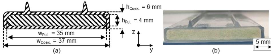
Figure 3: Cross-section area of the hybrid profile (a) and (b) photographic image.
