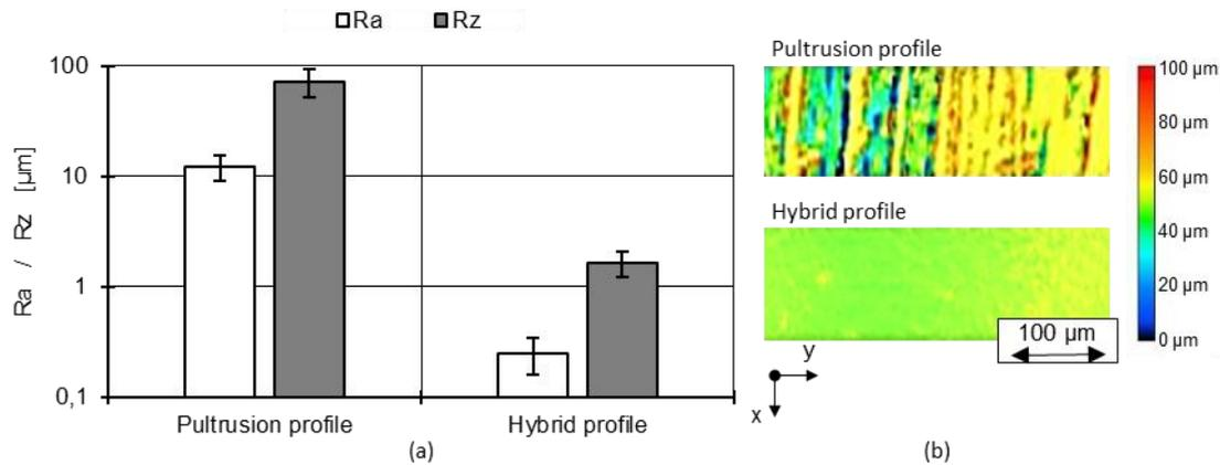
Figure 4: Average roughness of the pultruded profiles compared to hybrid PulEx profiles (a). Surface profiles recorded by LCM (b).
