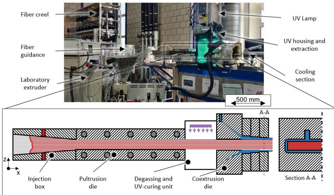
Figure 1: Process layout for the PulEx process (top) and sectional view of the tooling (bottom).
