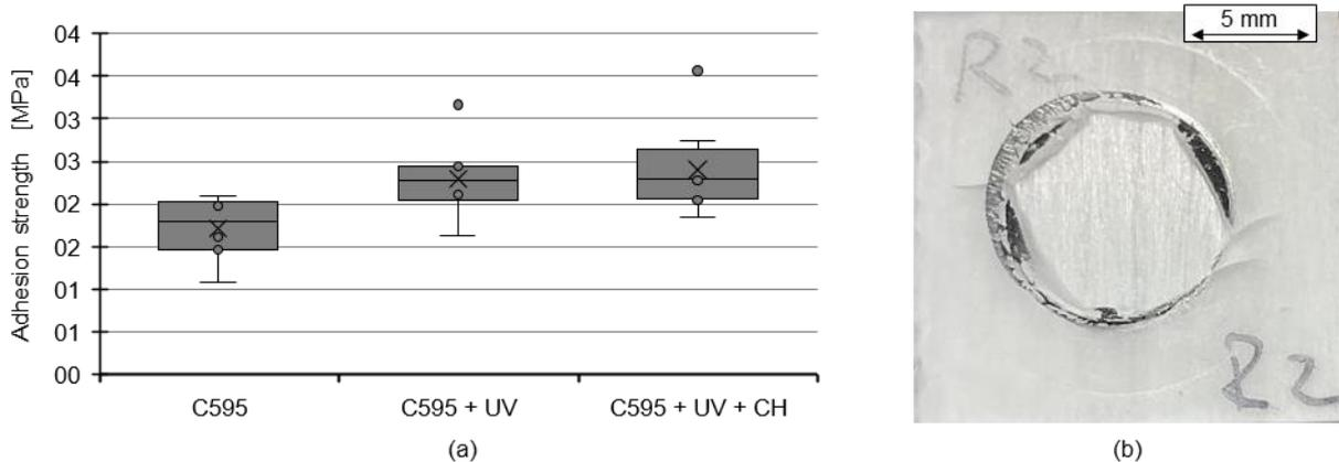
Figure 5: Adhesion strength of the surface coating and pultruded profile determined by LumiFrac measurements (a). In addition to the dual curing, convective heating (CH) by a heated air blower is performed. (b) shows the fractured surface. Black edges mark the remains of the adhesive.
