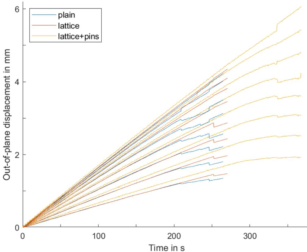
Figure 4: Out-of-plane displacement (evaluated by 3D-DIC, post-processed with *MATLAB*<sup>®</sup>) of 8 radial uniformly distributed points along a line on the top surfaces of the peeling specimens with different interface specifications until total failure.
