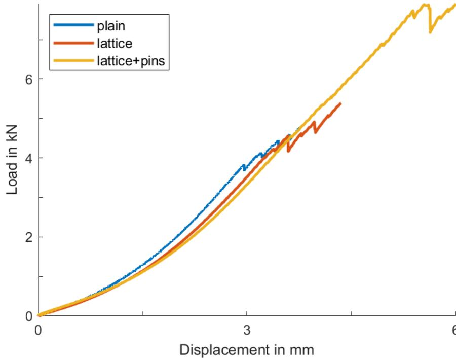
Figure 3: Load-displacement curves of peeling specimens with different interface specifications until total failure.
