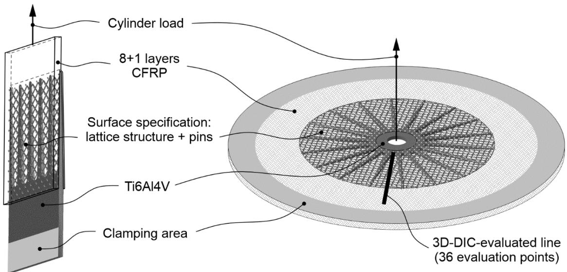
Figure 1: Left: Schematic of lap shear test specimen (Ti adherend: 80x25.4x1.5 mm);
