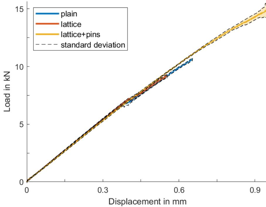
Figure 2: Load-displacement curves (mean value and standard deviation) of lap shear specimens with different interface specifications until total failure.
