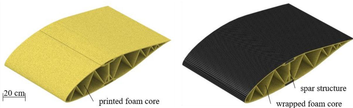
Figure 9: Foam structure of the optimised wing cross-section (left) and prototype component wrapped with carbon fibre fabric (right)
