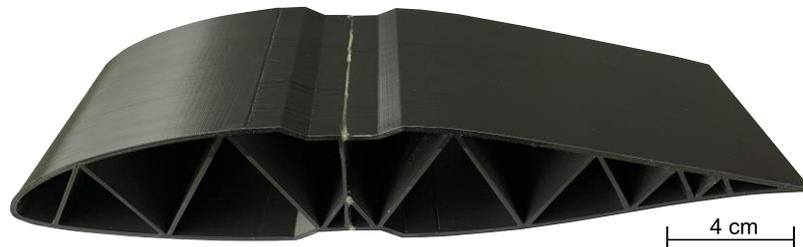
Figure 11: 3D-printed sample component of the concept wing cross-section
