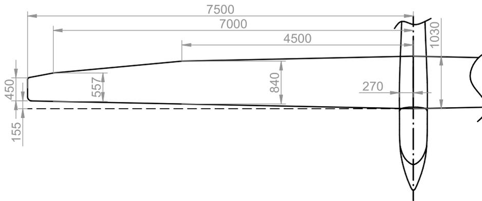
Figure 3: Geometry of the Astir wing [mm]
