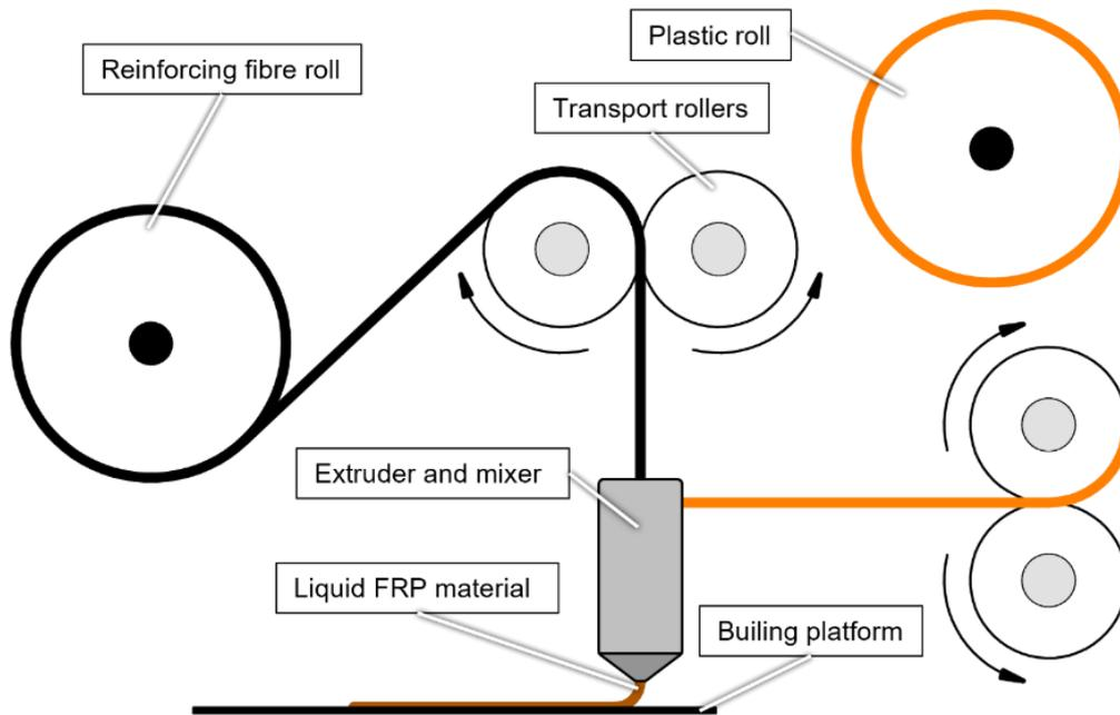
Figure 2: Principle sketch of the fibre integrated FDM printing process
