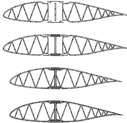
Figure 8: Procedure for producing the optimised wing cross-section
