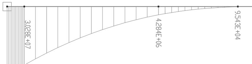
Figure 6: Bending moment [Nmm] over the wingspan
