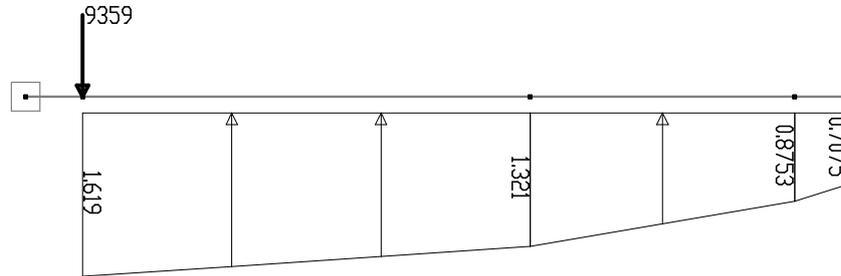
Figure 4: Mechanical system of the wing load: line loads [N/mm]; point load [N].
