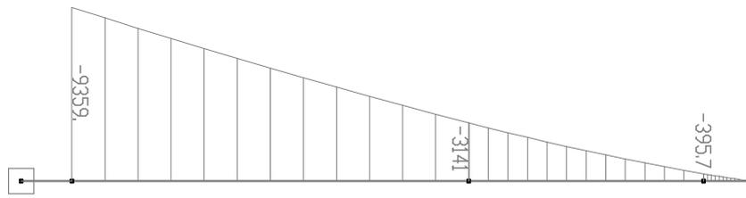
Figure 5: Shear force [N] over the wingspan
