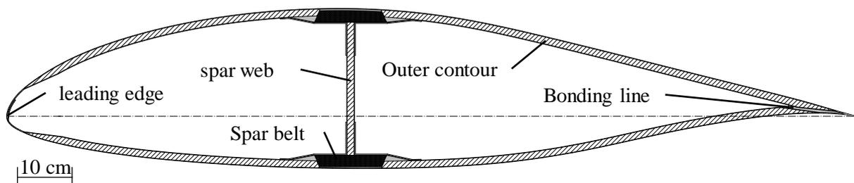
Figure 1: Cross section of a glider wing
