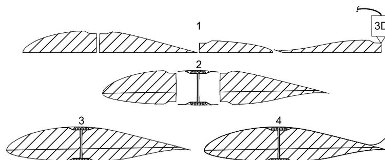
Figure 7: Procedure for producing the solid cross-section
