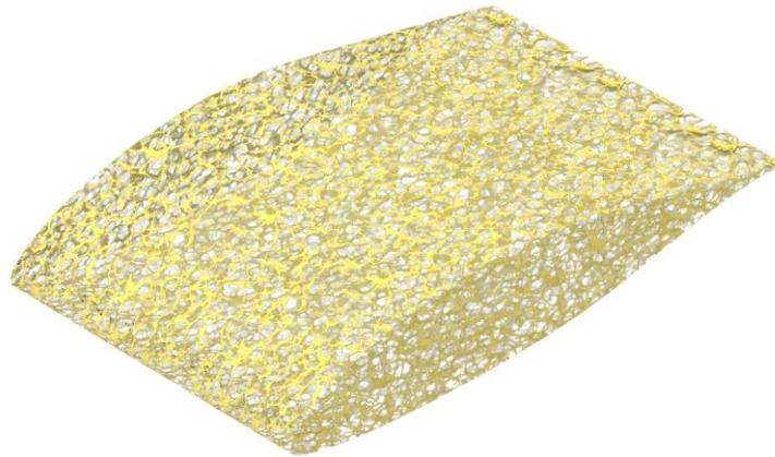
Figure 10: Innovative wing cross-section with bone-like foam structure
