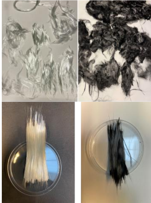
Figure 7: CF (left) and GF (right) type fibers retrieved from composite waste samples.
